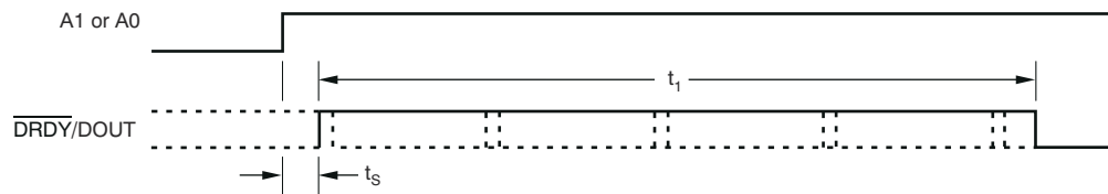
图 7-7. Example of Settling Time After Changing the Input Multiplexer
