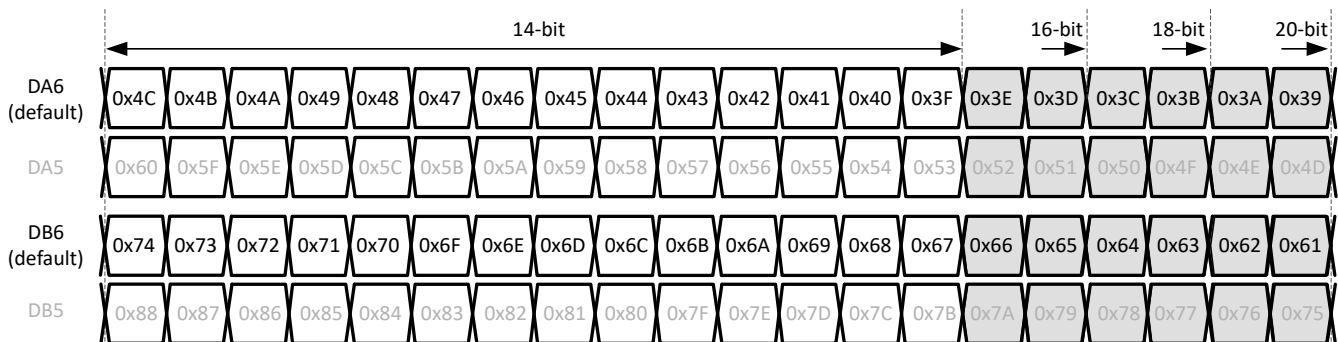
图 8-46. 1-wire output bit mapping
