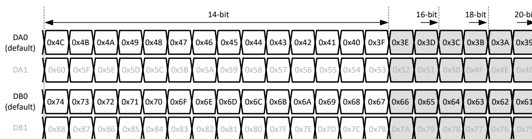
图 8-37. 1-wire output bit mapping
