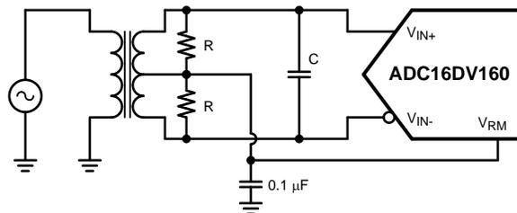
**Figure 28. Transformer Drive Circuit for Low Input Frequency**
