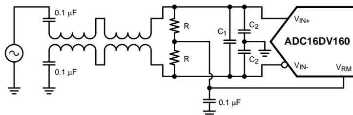
**Figure 29. Transformer Drive Circuit for High Input Frequency**
