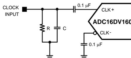
**Figure 34. Singled-Ended 1.8V Clocking, Capacitive AC Coupled**
