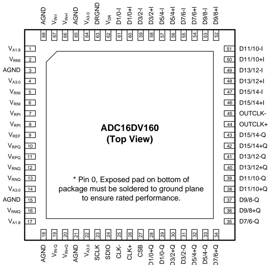
Figure 2. Pin-Out of ADC16DV160
