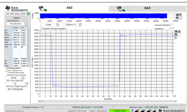
图 8-6. 40-MHz, Square-Wave Time Domain for 5-GSPS, Single-Channel Oscilloscope
