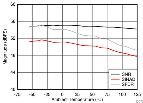
JMODE 1, BG calibration,  $f_s = 6400\text{ MSPS}$ ,  $f_{\text{IN}} = 2482\text{ MHz}$ ,
