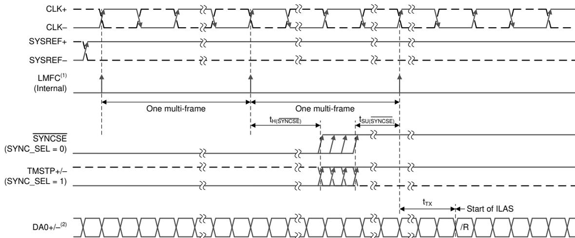
A. It is assumed that the internal LMFC is aligned with the rising edge of CLK± that captures the SYSREF± high value.
