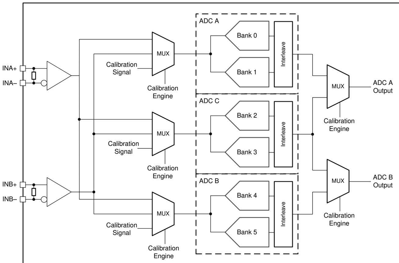
图 7-23. ADC12DJ3200QML-SP Calibration System Block Diagram
