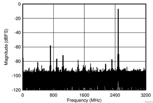
JMODE 1, FG calibration,  $f_s = 6400\text{ MSPS}$ ,  $f_1 = 2477\text{ MHz}$ ,  $f_2 = 2487\text{ MHz}$ ,  $A_{\text{IN}} = -7\text{ dBFS}$  per tone, SFDR =  $-58\text{ dBFS}$ , IMD3 =  $-70\text{ dBFS}$ , IMD2 =  $-75\text{ dBFS}$
