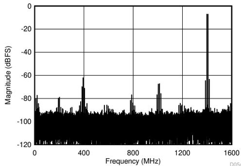
JMODE 3, FG calibration,  $f_s = 3200\text{ MSPS}$ ,  $f_1 = 4992\text{ MHz}$ ,  $f_2 = 5002\text{ MHz}$ ,  $A_{\text{IN}} = -7\text{ dBFS}$  per tone, SFDR =  $-62\text{ dBFS}$ , IMD3 =  $-63\text{ dBFS}$ , IMD2 =  $-80\text{ dBFS}$
