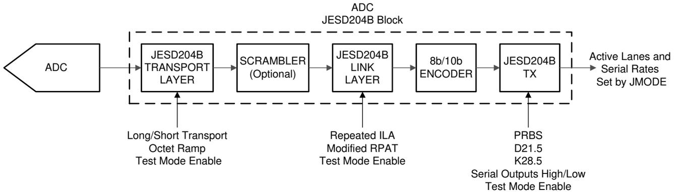
图 7-22. Test Mode Insertion Points
