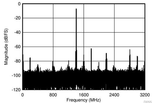
JMODE 1, FG calibration,  $f_s = 6400\text{ MSPS}$ ,  $f_1 = 4992\text{ MHz}$ ,  $f_2 = 5002\text{ MHz}$ ,  $A_{\text{IN}} = -7\text{ dBFS}$  per tone, SFDR =  $-62\text{ dBFS}$ , IMD3 =  $-65\text{ dBFS}$ , IMD2 =  $-71\text{ dBFS}$
