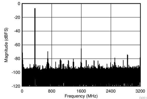
JMODE 1, FG calibration,  $f_s = 6400\text{ MSPS}$ ,  $f_1 = 342\text{ MHz}$ ,  $f_2 = 352\text{ MHz}$ ,  $A_{\text{IN}} = -7\text{ dBFS}$  per tone, SFDR =  $-70\text{ dBFS}$ , IMD3 =  $-91\text{ dBFS}$ , IMD2 =  $-71\text{ dBFS}$
