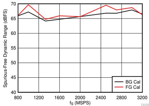
JMODE 3, FG and BG calibration,  $f_{IN} = 2482\text{ MHz}$ ,  $A_{IN} = -1\text{ dBFS}$
