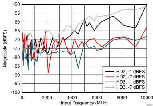
JMODE 3,  $f_s = 3200\text{ MHz}$ , FG calibration
