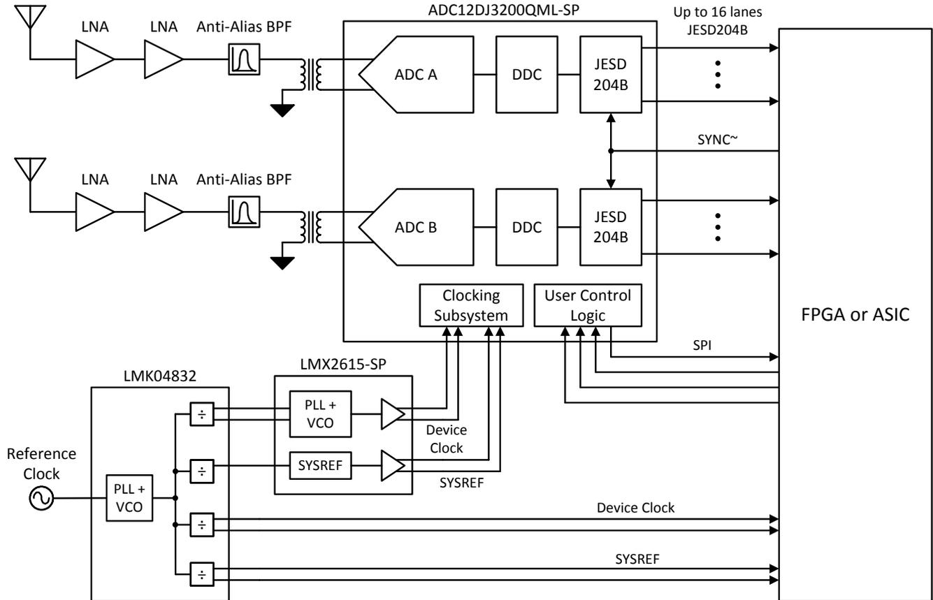
图 8-1. Typical Configuration for Wideband RF Sampling Receiver
