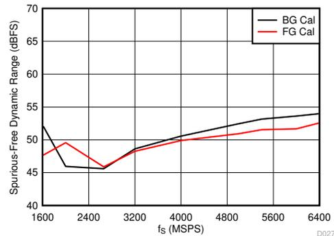
JMODE 1, FG and BG calibration,  $f_{IN} = 2482\text{ MHz}$ ,  $A_{IN} = -1\text{ dBFS}$
