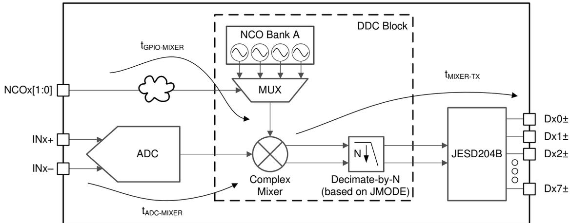
图 7-6. NCO Fast Frequency Hopping Latency Diagram
