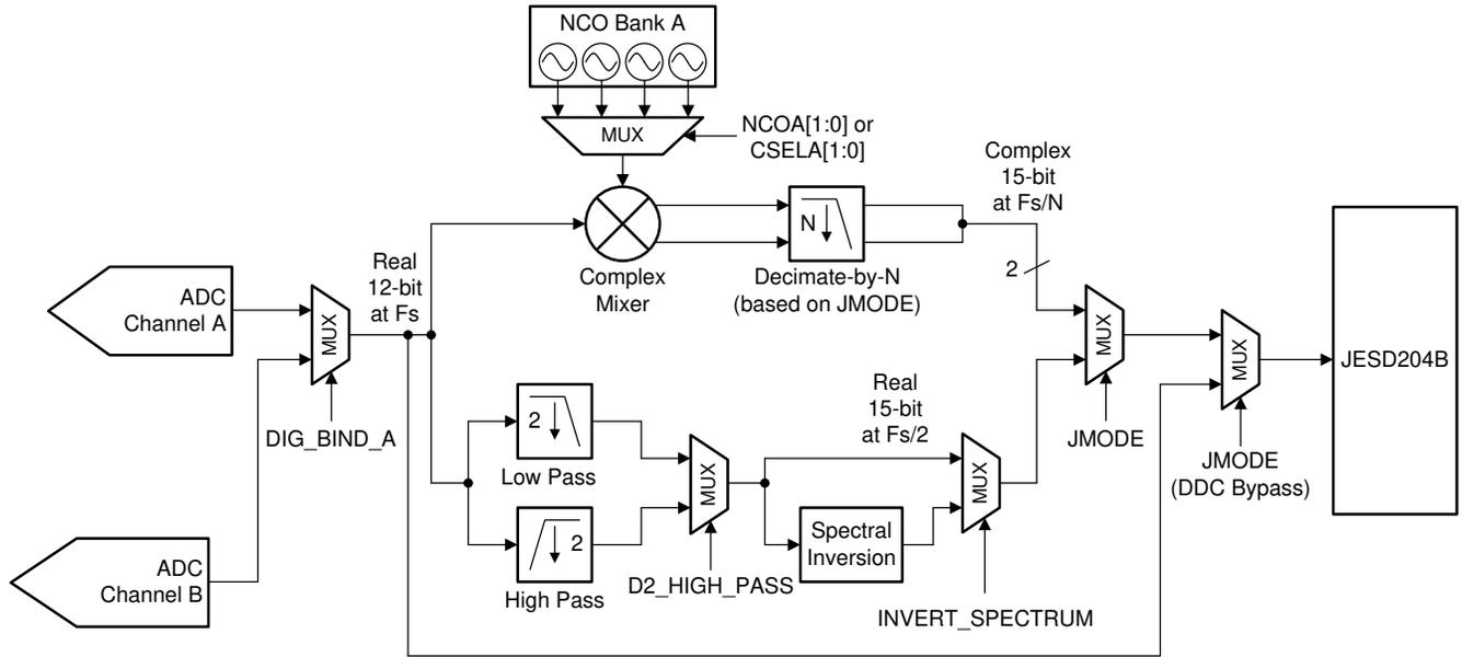
图 7-5. Channel A Digital Down Conversion Block (Dual-Channel Mode Only)
