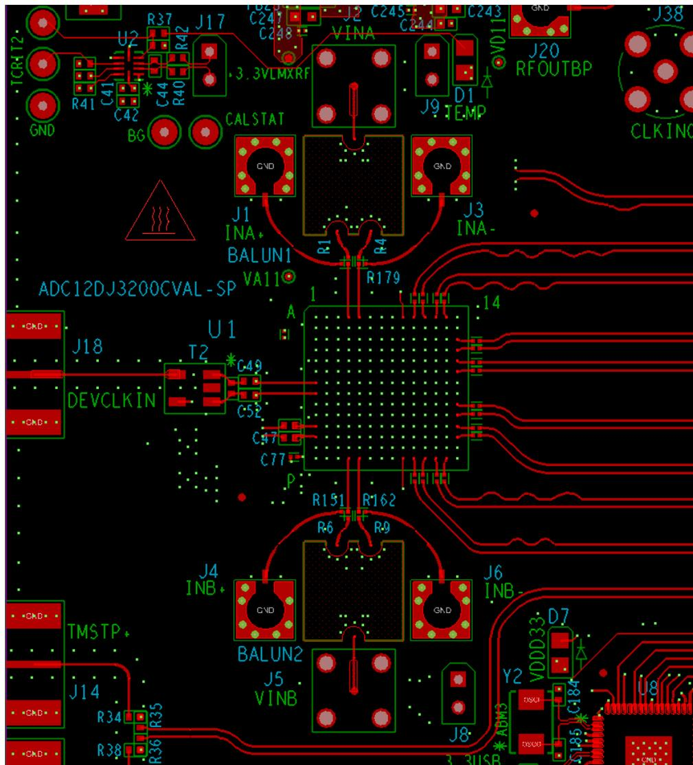
图 9-1. Top Layer Routing: Analog Inputs, CLK and SYSREF, DA0-3, DB0-3
