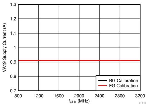
JMODE 1,  $f_{\text{IN}} = 2482\text{ MHz}$ ,  $A_{\text{IN}} = -1\text{ dBFS}$
