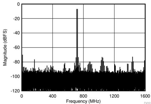
JMODE 3, FG calibration,  $f_s = 3200\text{ MSPS}$ ,  $f_1 = 2477\text{ MHz}$ ,  $f_2 = 2487\text{ MHz}$ ,  $A_{\text{IN}} = -7\text{ dBFS}$  per tone, SFDR =  $-70\text{ dBFS}$ , IMD3 =  $-74\text{ dBFS}$ , IMD2 =  $-70\text{ dBFS}$
