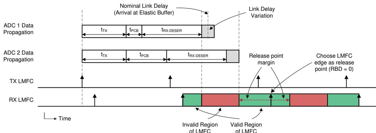
**图 7-20. LMFC Valid Region Definition for Elastic Buffer Release Point Selection**
