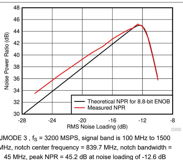
**图 8-3. NPR vs Input RMS Noise Loading in Dual-Channel Mode**
