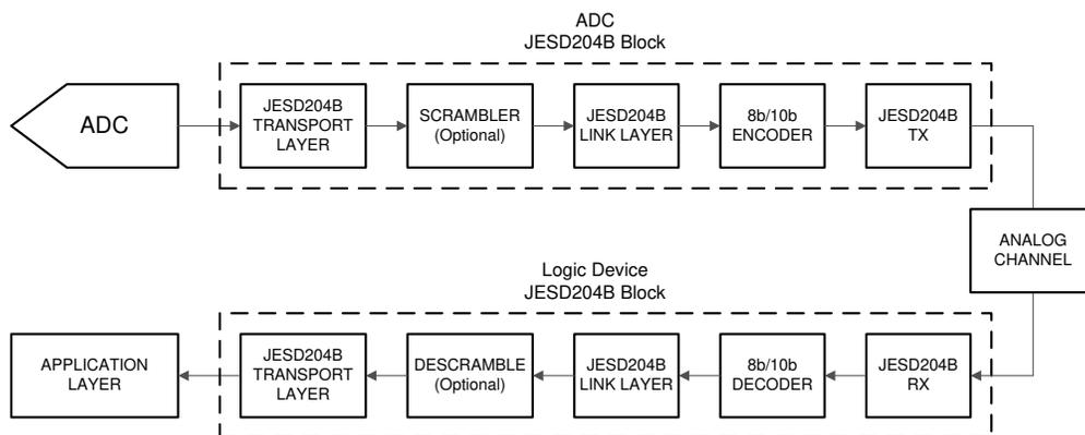
图 7-19. Simplified JESD204B Interface Diagram
