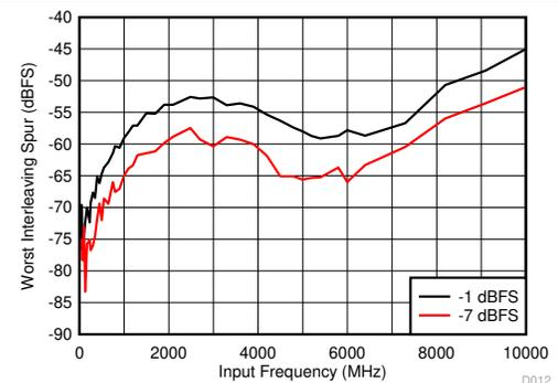
JMODE 1,  $f_s = 6400\text{ MHz}$ , FG calibration, includes  $f_s / 2 - f_{\text{IN}}$  and  $f_s / 4 \pm f_{\text{IN}}$  spurs only
