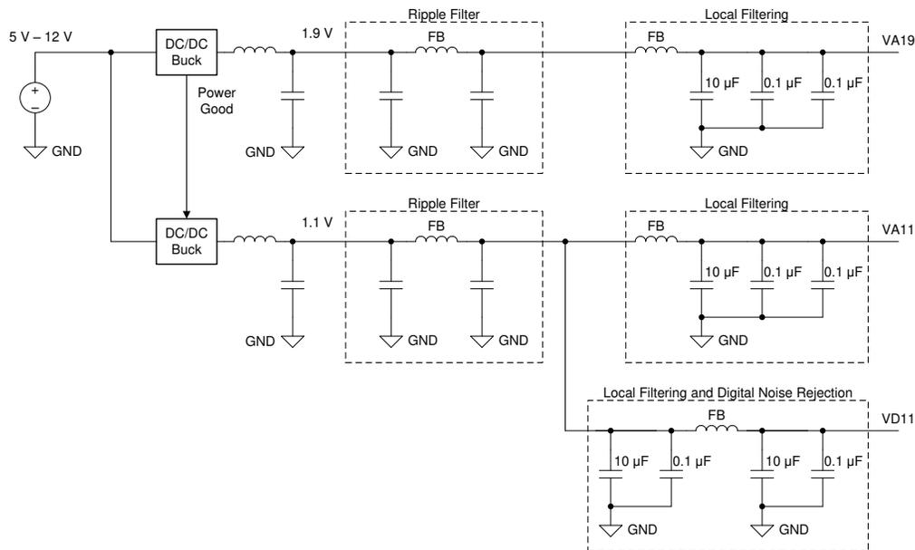
图 9-2. DC/DC Switching Regulator Example
