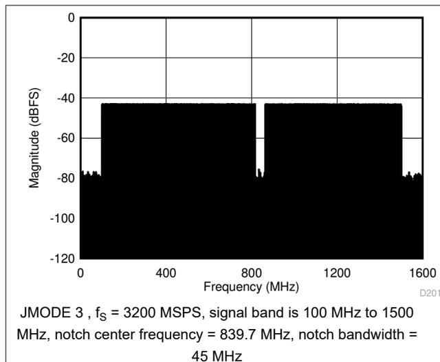
**图 8-2. Example NPR Measurement at Optimal Loading for ADC12DJ3200QML-SP in Dual-Channel Mode**
