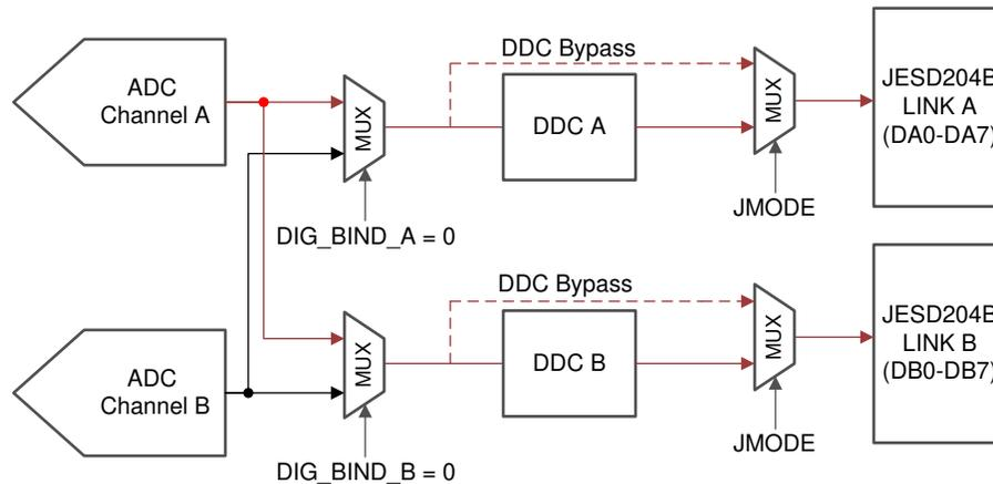
图 7-21. Dual DDC Mode or Redundant Data Mode for Channel A
