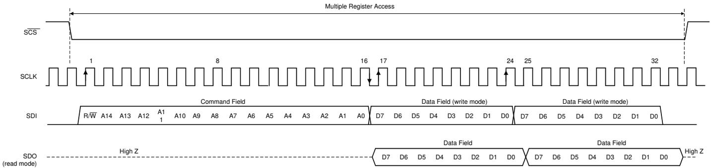
**Figure 7-25. Serial Interface Protocol: Streaming Read and Write**
