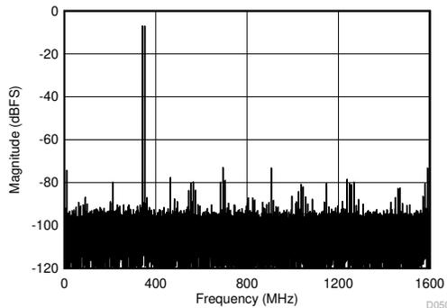
JMODE 3, FG calibration,  $f_s = 3200\text{ MSPS}$ ,  $f_1 = 342\text{ MHz}$ ,  $f_2 = 352\text{ MHz}$ ,  $A_{\text{IN}} = -7\text{ dBFS}$  per tone, SFDR =  $-73\text{ dBFS}$ , IMD3 =  $-87\text{ dBFS}$ , IMD2 =  $-74\text{ dBFS}$
