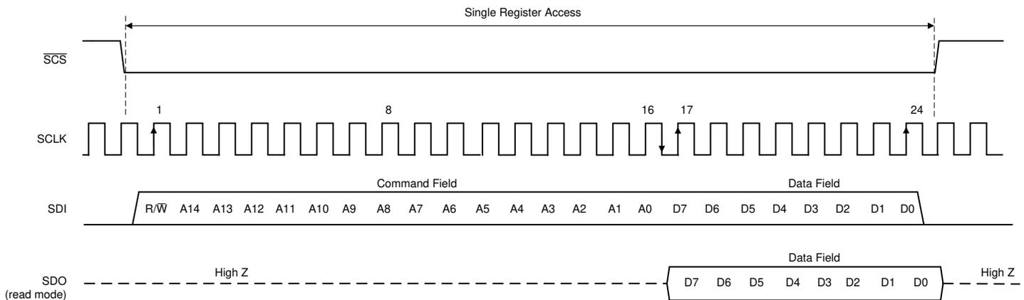
**图 7-24. Serial Interface Protocol: Single Read/Write**
