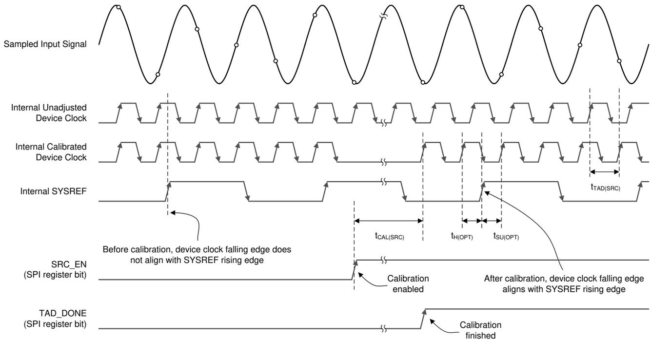
图 7-4. SYSREF Calibration Timing Diagram
