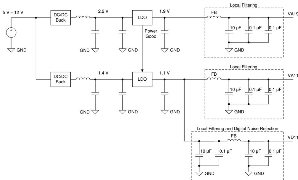
**图 9-1. LDO Linear Regulator Example**
