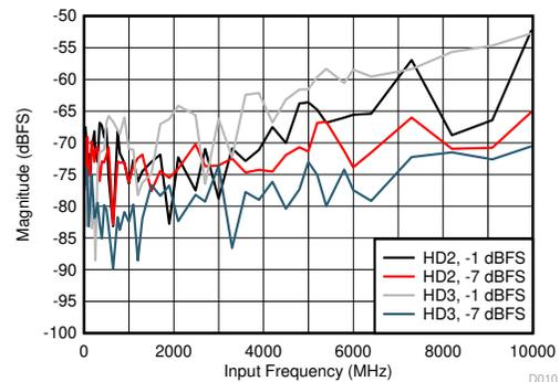
JMODE 1,  $f_s = 6400\text{ MHz}$ , FG calibration
