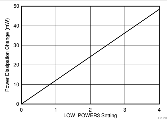
图 7-13. Power Dissipation Change vs LOW_POWER3 register setting
