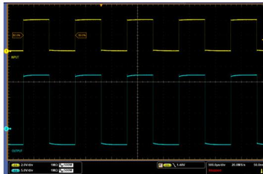
图 8-18. PWM Input (yellow) and Driver Output (blue)
