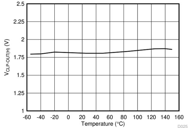
图 5-19.  $V_{CLP-OUT(H)}$  Short Circuit Clamping Voltage vs Temperature
