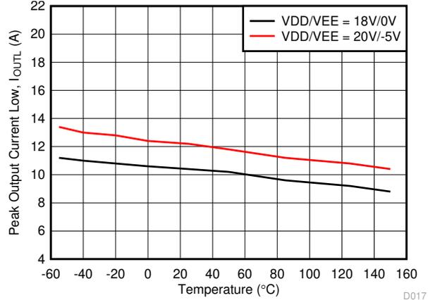
图 5-5. Output Low Driver Current vs Temperature
