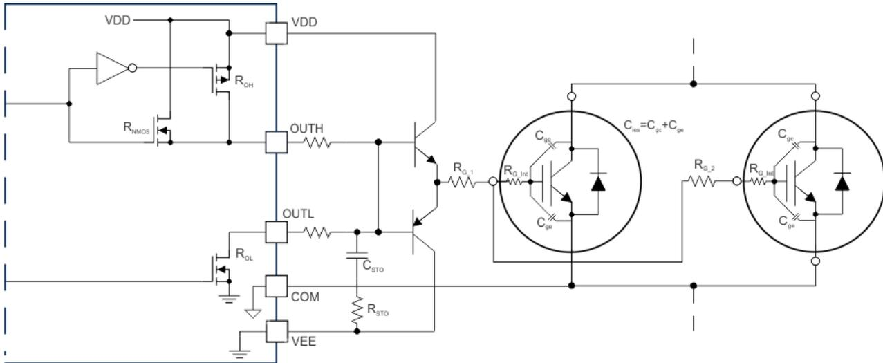
图 8-17. Current Buffer for Increased Drive Strength
