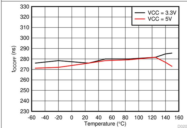
图 5-24.  $t_{OCOFF}$  OC Propagation Delay vs Temperature
