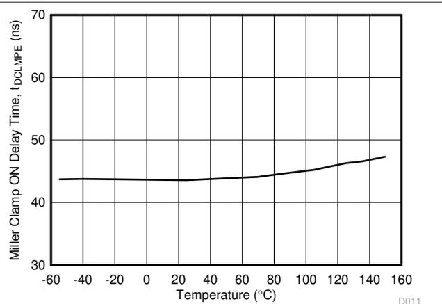
图 5-23.  $t_{DCLMPE}$  Miller Clamp ON Delay Time vs Temperature
