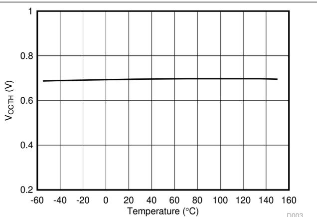
图 5-25.  $V_{OCTH}$  OC Detection Threshold vs Temperature
