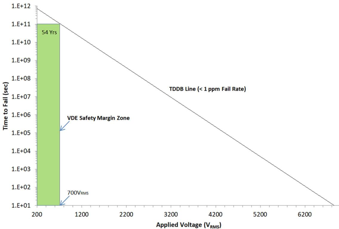
图 5-3. Basic Isolation Capacitor Life Time Projection
