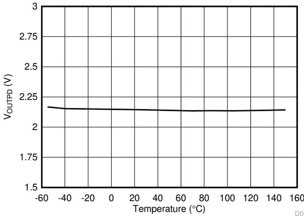
图 5-18.  $V_{OUTPD}$  Output Active Pulldown Voltage vs Temperature
