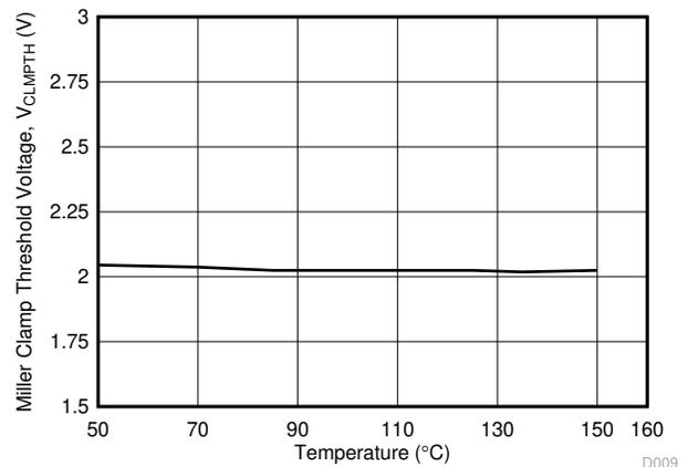
图 5-21.  $V_{CLMPH}$  Miller Clamp Threshold Voltage vs Temperature
