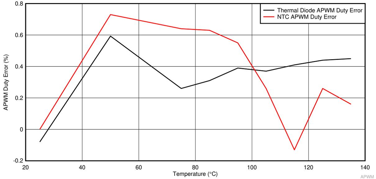
图 8-15. APWM Duty Error with Single-Point Calibration
