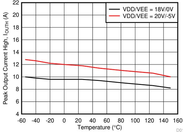
图 5-4. Output High Drive Current vs Temperature
