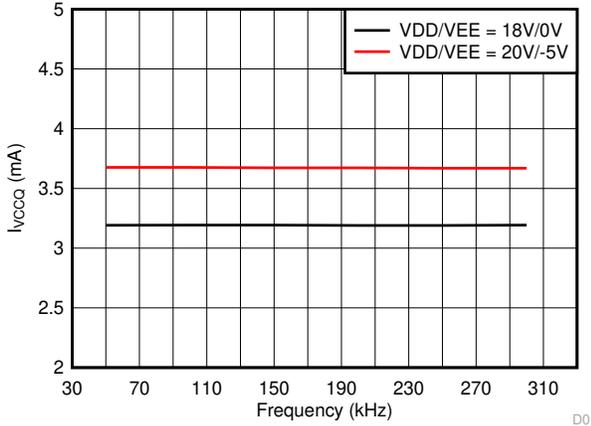
图 5-8. I<sub>VCCQ</sub> Supply Current vs Input Frequency
