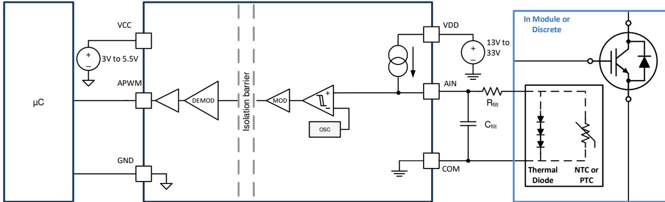
图 8-11. Thermal Diode or Thermistor Temperature Sensing Configuration
