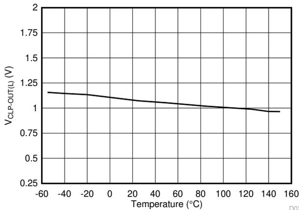
图 5-20.  $V_{CLP-OUT(L)}$  Short Circuit Clamping Voltage vs Temperature
