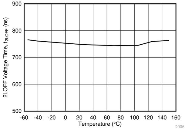
图 5-28. t<sub>2LOFF</sub> 2-Level Turn Off Time vs Temperature
