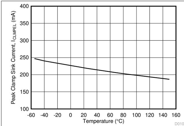
图 5-22.  $I_{CLMPEL}$  Miller Clamp Sink Current vs Temperature
