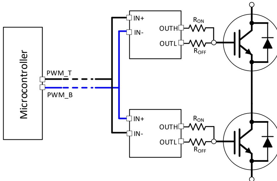
图 8-2. PWM Interlock for a Half Bridge
