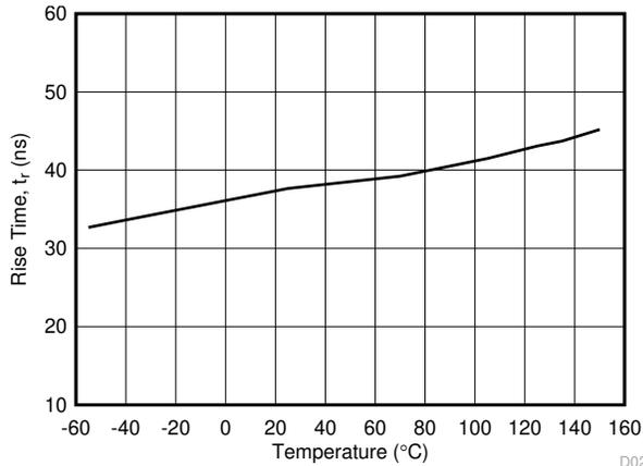
$V_{CC} = 3.3V$        $V_{DD} = 18V$        $C_L = 10nF$
