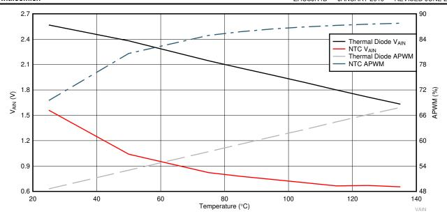
图 8-12. Thermal diode and NTC  $V_{AIN}$  and Corresponding Duty Cycle at APWM
