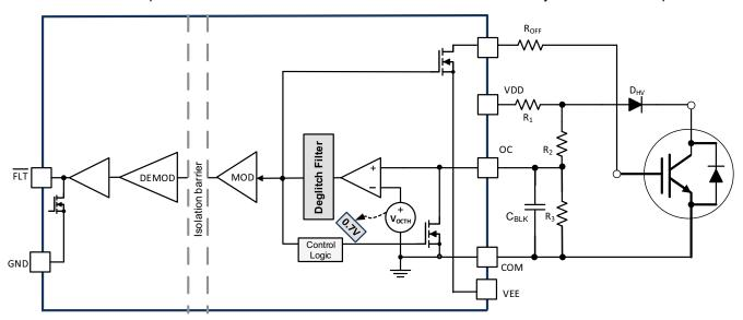
图 8-8. Overcurrent and Short Circuit Protection Based on Desaturation Circuit
