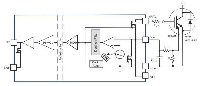
图 8-7. Overcurrent and Short Circuit Protection Based on IGBT Module with SenseFET
