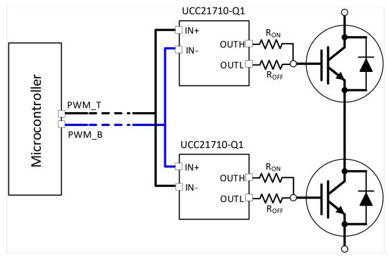
图 8-2. PWM Interlock for a Half Bridge
