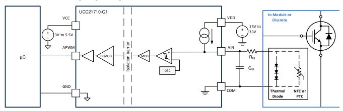
图 7-7. Isolated Analog to PWM Signal
