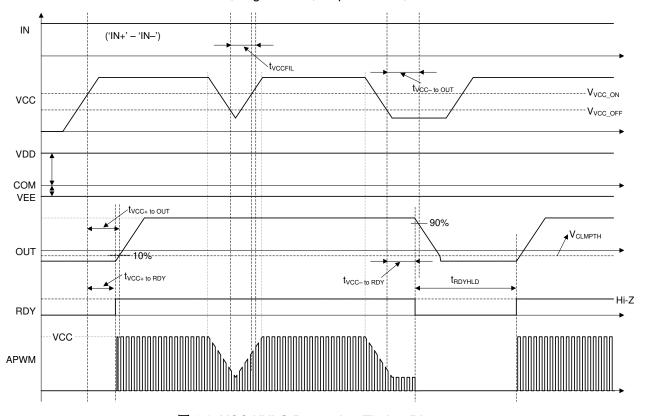
图 6-8. VCC UVLO Protection Timing Diagram
