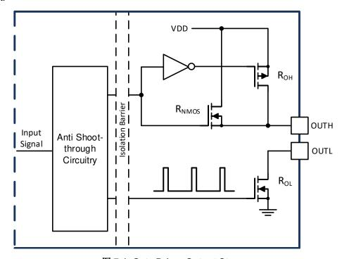
图 7-1. Gate Driver Output Stage
