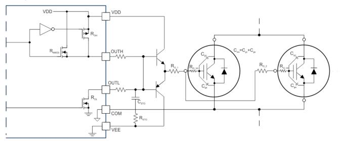
图 8-16. Current Buffer for Increased Drive Strength
