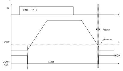
图 6-7. Timing Diagram for Internal Active Miller Clamp Function
