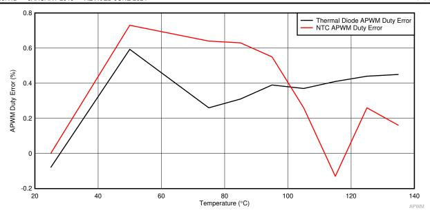
图 8-14. APWM Duty Error with Single-Point Calibration
