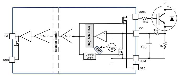
图 7-5. Overcurrent and Short Circuit Protection
