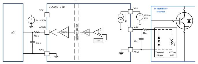
图 8-11. APWM Channel with Filtered Output
