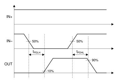
图 6-2. Inverting Logic Propagation Delay Measurement
