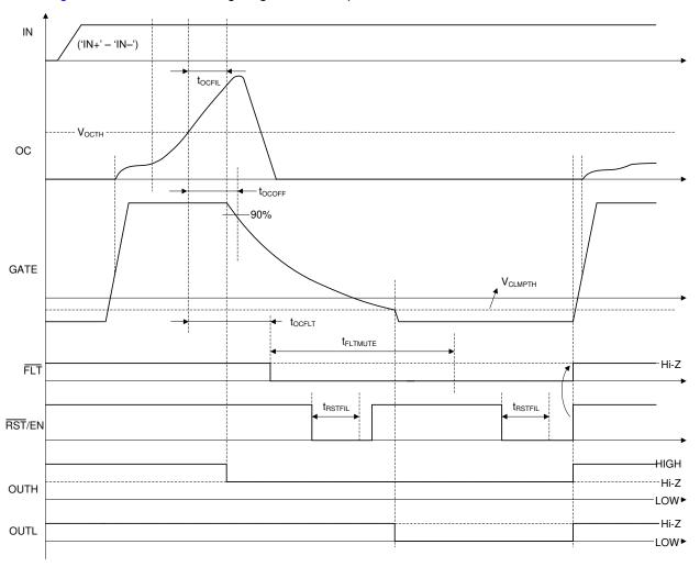
图 6-10. OC Protection with Soft Turn-OFF
