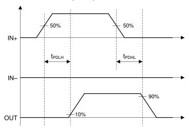
图 6-1. Non-inverting Logic Propagation Delay Measurement
