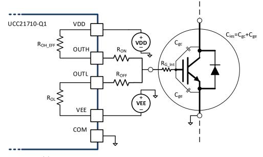
图 8-5. Output Model for Calculating Peak Gate Current
