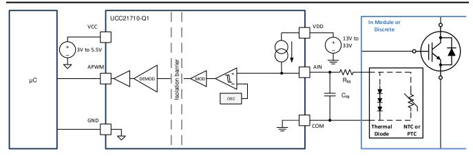
图 8-10. Thermal Diode or Thermistor Temperature Sensing Configuration
