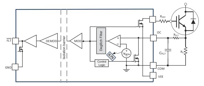
图 8-9. Overcurrent and Short Circuit Protection Based on Shunt Resistor
