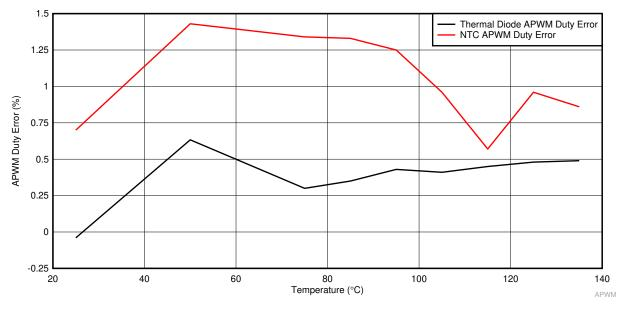
图 8-13. APWM Duty Error Without Calibration
