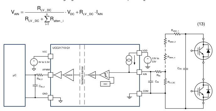
图 8-15. DC-link Voltage Sensing Configuration
