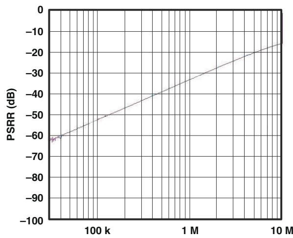
图 6-16. Com Port to No0 PSRR,  $In1 = V_{CC}$ ,  $In2 = V_{CC}$  ( $V_{CC} = 5$  V)
