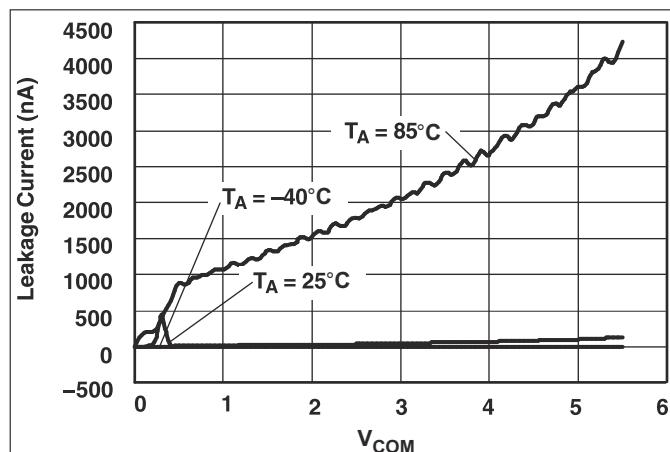
图 6-7. I<sub>COM(PWROFF)</sub> Leakage Current vs V<sub>COM</sub> Over Temperature (V<sub>CC</sub> = 0 V)
