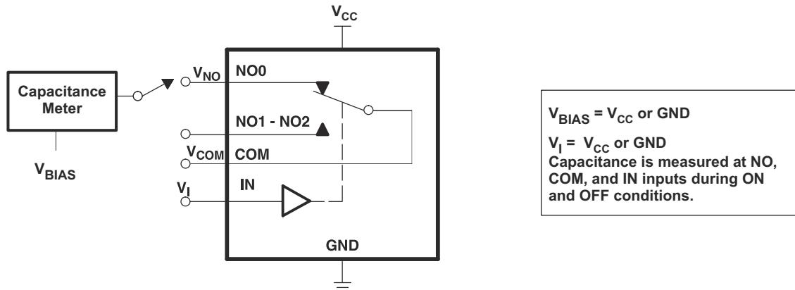
图 7-4. Capacitance ( $C_I$ ,  $C_{COM(ON)}$ ,  $C_{NO(OFF)}$ ,  $C_{COM(OFF)}$ ,  $C_{NO(ON)}$ )
