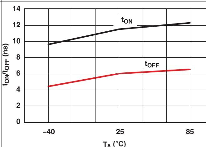
图 6-10. T<sub>ON</sub> and T<sub>OFF</sub> vs Temperature
