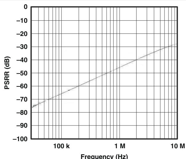
图 6-17. Com Port Hi-Z PSRR,  $In1 = 0$  V,  $In2 = 0$  V ( $V_{CC} = 5$  V)
