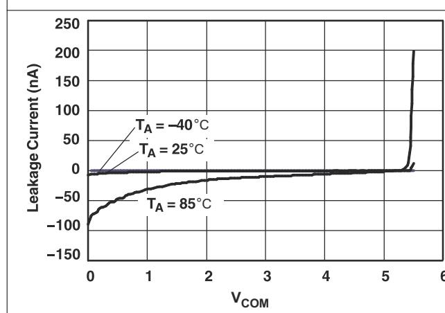
图 6-5.  $I_{NO(OFF)}$  Leakage Current vs  $V_{COM}$  Over Temperature ( $V_{CC} = 5\text{ V}$ )
