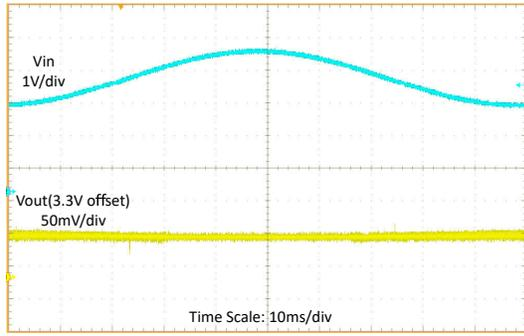
$V_{IN} = 2.7V$  至  $4.3V$  扫描,  $I_{OUT} = 1A$
