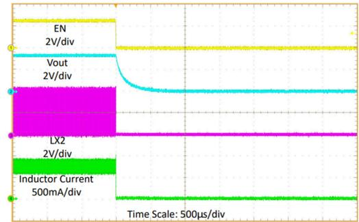
$V_{IN} = 3.6V$ ,  $V_{OUT} = 3.3V$   $R_{load} = 4\Omega$ , MODE = 低电平
