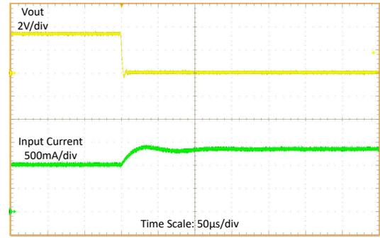
$V_{IN} = 3.6V$ ,  $V_{OUT} = 3.3V$   $I_{OUT} = 1A$ , FPWM
