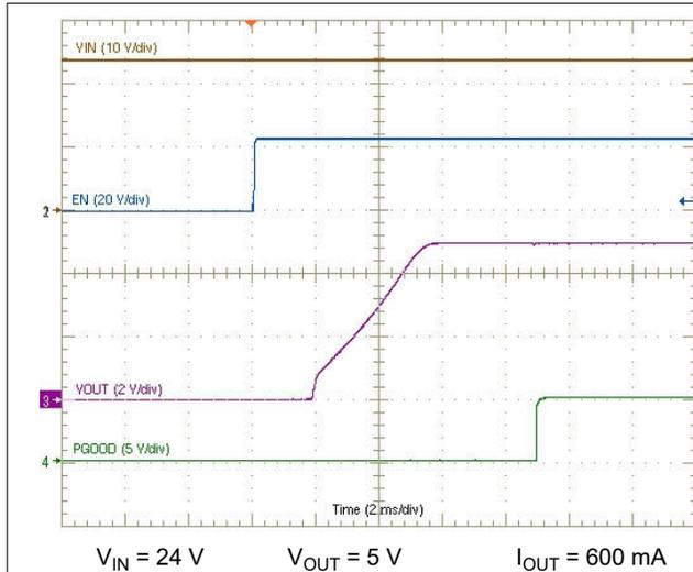
图 8-2. Start-Up Waveforms
