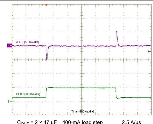
图 8-5. Transient Response Waveform
