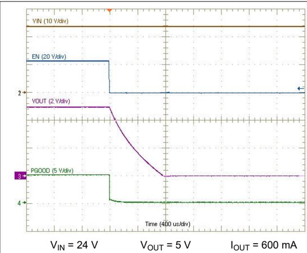
图 8-3. Enable Shutdown Waveforms
