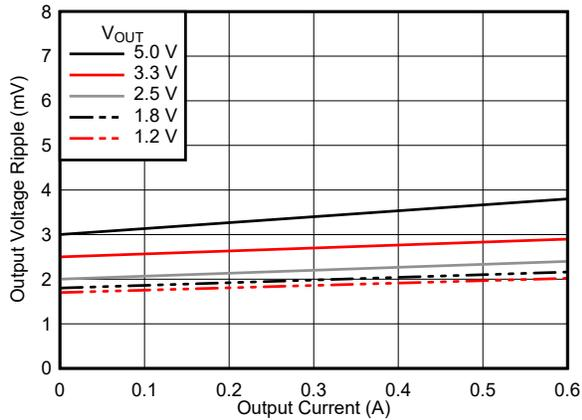
$C_{OUT} = 4 \times 47\ \mu\text{F}$ , 25-V, ceramic
