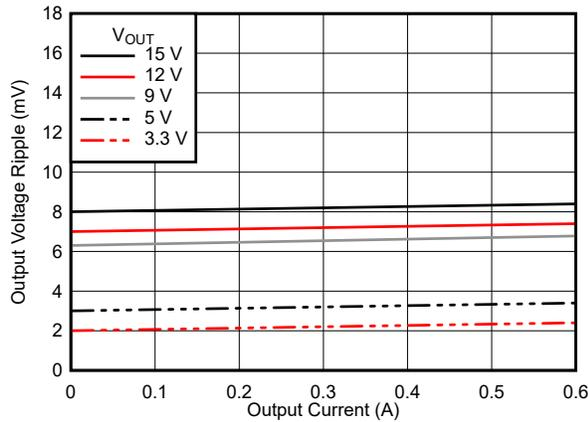
$C_{OUT} = 2 \times 47\text{-}\mu\text{F}$ , 25-V, ceramic
