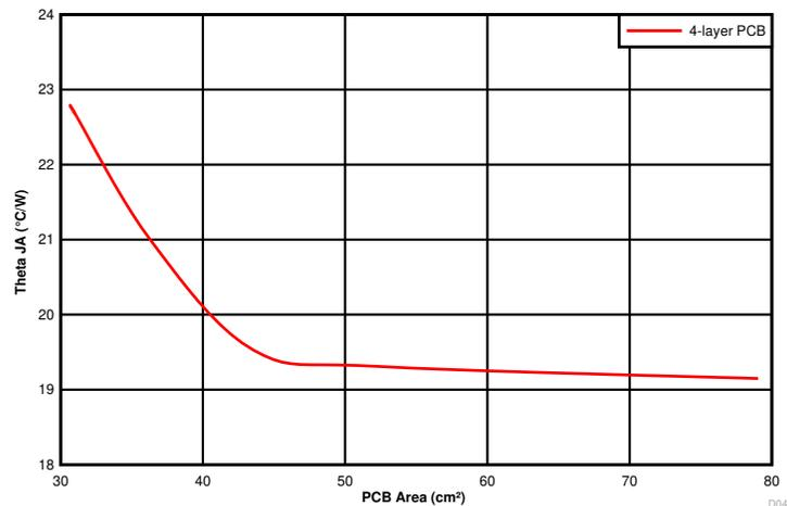
图 10-4.  $R_{\theta JA}$  versus PCB Area (per Layer)
