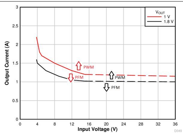
图 7-15. PFM/PWM Thresholds (1 V and 1.8 V)
