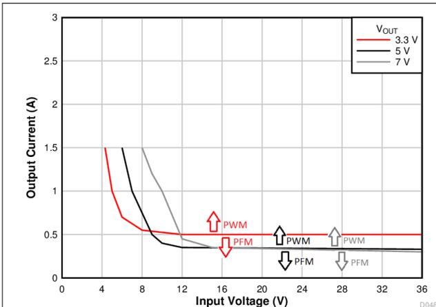
图 7-14. PFM/PWM Thresholds (3.3 V, 5 V, and 7 V)
