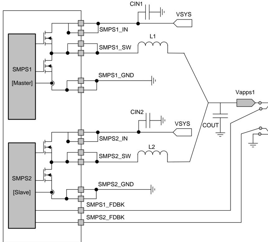
图 5-14. SMPS1&2 Dual-Phase Configuration
