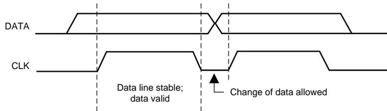
图 5-18. Bit Transfer on the Serial Interface
