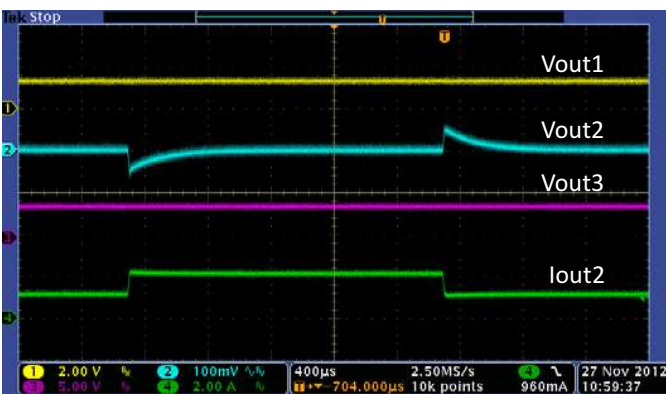
Figure 23. Transient Response Buck2@1.8V, 1-2A Step, C_o = 47\mu\text{F}
