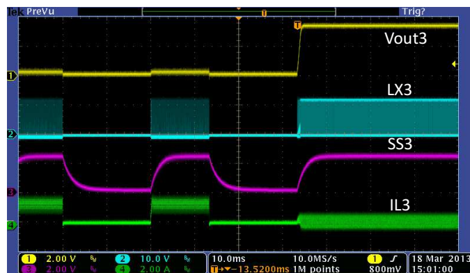
Figure 36. Hiccup Recover, Buck3=3.3V
