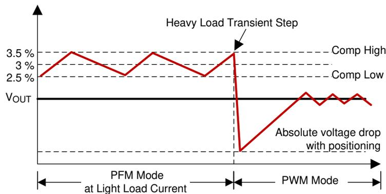
图 8-4. Power-Save Mode Thresholds and Dynamic Voltage Positioning
