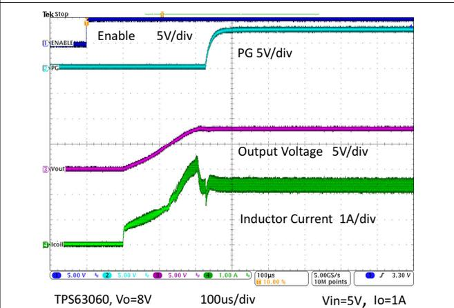
图 9-23. Startup After Enable
