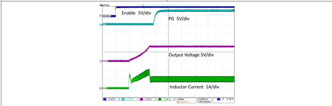
图 9-24. Startup After Enable
