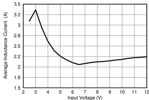
**图 8-5. Average Inductance Current vs Input Voltage**
