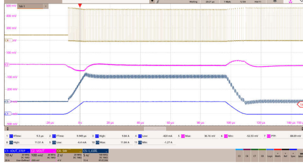
V_{IN} = 5.0V TPS6286A10 BOM = 4 \times 22 \mu F V_{OUT} = 0.9V I_{OUT} = 10mA \text{ 至 } 10A
