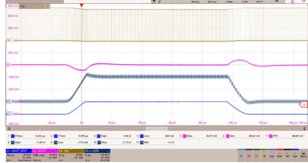
V_{IN} = 5.0V TPS6286A10 BOM = 4 \times 22 \mu F V_{OUT} = 0.9V I_{OUT} = 10mA \text{ 至 } 10A
