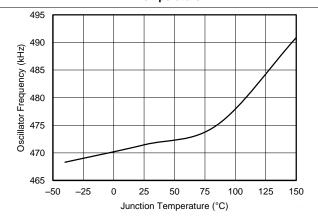
Figure 4. Oscillator Frequency vs Junction Temperature
