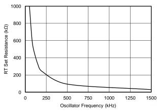
Figure 16. RT Set Resistor vs Switching Frequency
