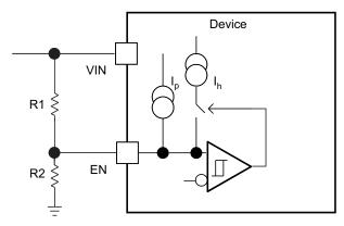
Figure 15. Adjustable VIN Undervoltage Lockout
