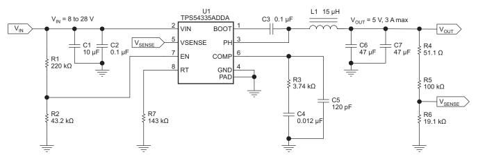
Figure 22. Typical Application Schematic, TPS54335A and TPS54335-1A
