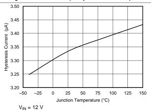
Figure 6. Hysteresis Current vs Junction Temperature
