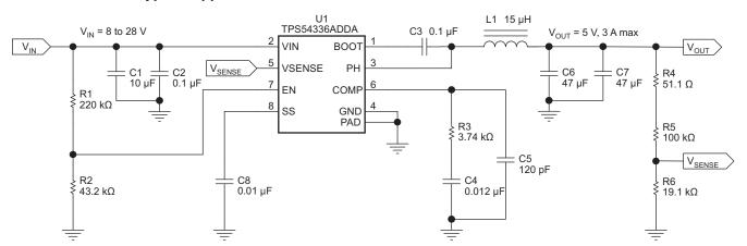
Figure 38. Typical Application Schematic, TPS54336A
