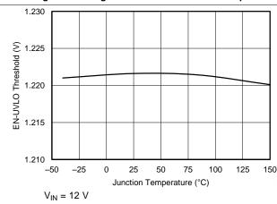
Figure 5. UVLO Threshold vs Junction Temperature
