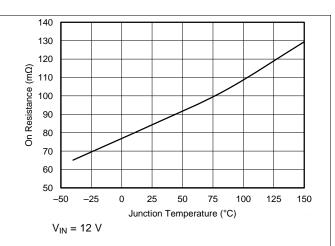
Figure 2. Low-Side MOSFET on Resistance vs Junction Temperature
