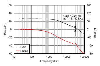
Figure 23. Power Stage Gain and Phase Characteristics
