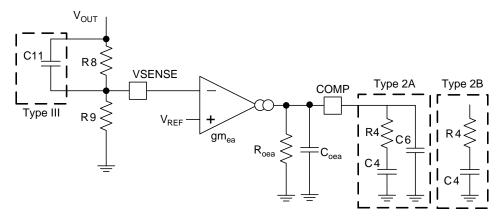
Figure 20. Types of Frequency Compensation
