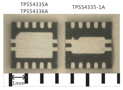
Figure 21. Difference Between the Two DRC Packages
