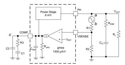
Figure 17. Small-Signal Model For Loop Response
