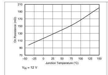
Figure 1. High-Side MOSFET on Resistance vs Junction Temperature
