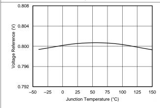
Figure 3. Voltage Reference vs Junction Temperature
