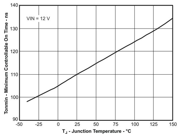
**图 6-5. Minimum Controllable on Time vs Junction Temperature**
