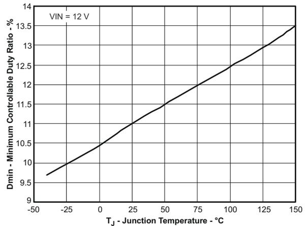
**图 6-6. Minimum Controllable Duty Ratio vs Junction Temperature**
