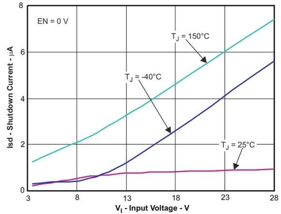
**图 6-2. Shutdown Quiescent Current vs Input Voltage**
