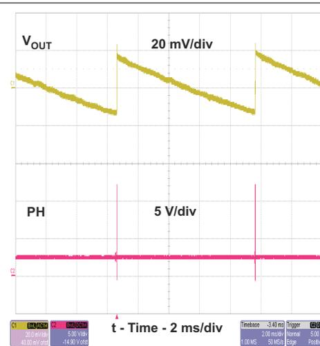
**图 8-11. TPS54332 Output Ripple during Eco-mode Operation**
