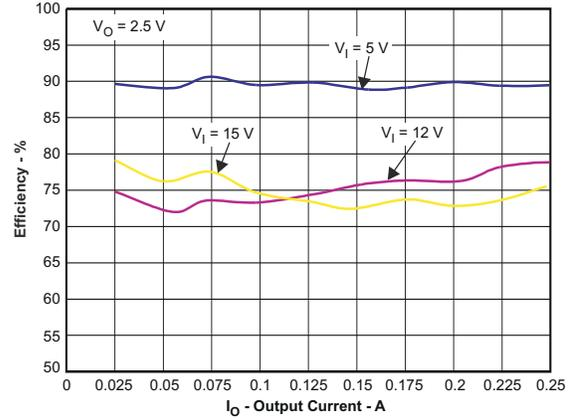
图 8-3. TPS54332 Low-Current Efficiency
