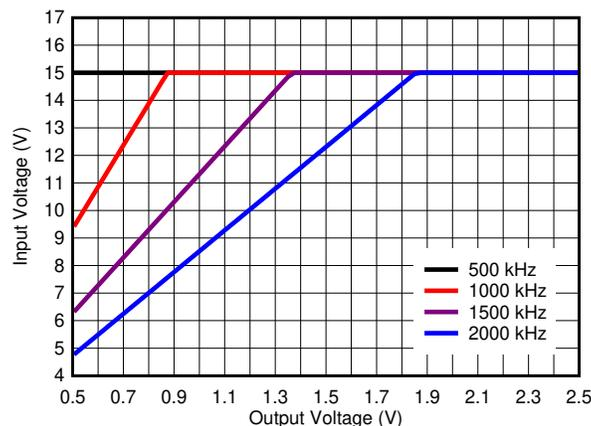
图 8-2. Maximum Input Voltage Versus Output Voltage
