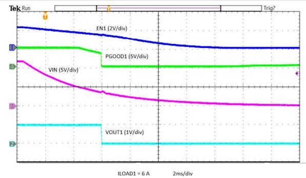
图 8-24. Power Down with  $V_{IN}$   $V_{OUT1}$
