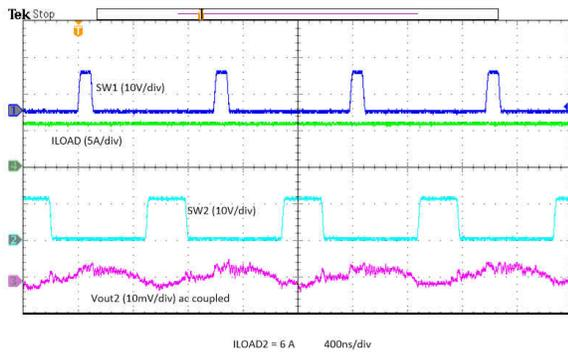
图 8-29.  $V_{OUT2}$  Output Ripple - 6-A Load
