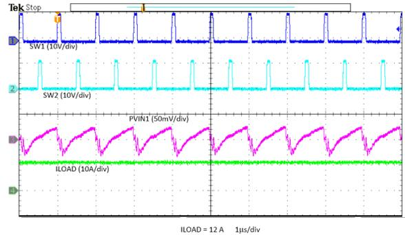
图 8-47. Input Ripple PVIN1 - 12-A Load
