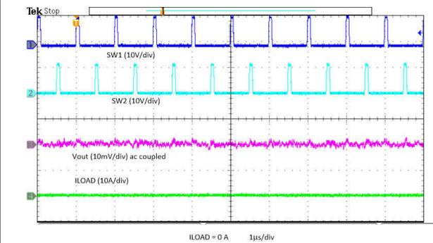
图 8-45. Output Ripple - No Load
