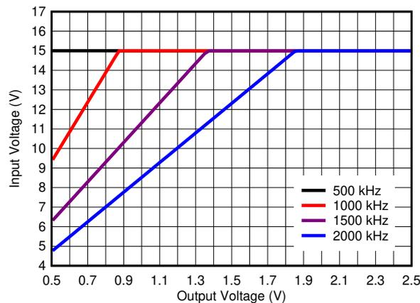
图 8-33. Maximum Input Voltage Versus Output Voltage
