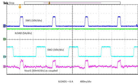
图 8-28.  $V_{OUT1}$  Output Ripple - 6-A Load
