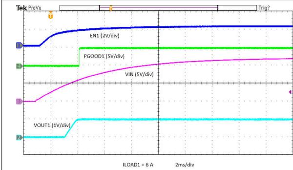
图 8-23. Power Up with  $V_{IN}$   $V_{OUT1}$
