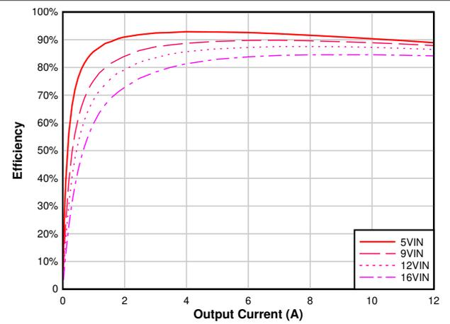
**图 6-2. Efficiency vs Output Current,  $V_{OUT} = 1.8\text{ V}$ ,  $F_{SW} = 1\text{ MHz}$**
