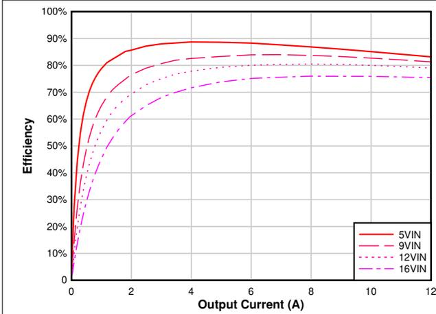
**图 6-1. Efficiency vs Output Current,  $V_{OUT} = 1.0\text{ V}$ ,  $F_{SW} = 1\text{ MHz}$**
