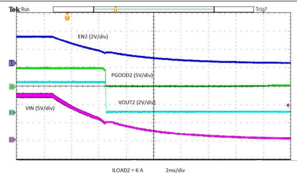
图 8-26. Power Down with  $V_{IN}$   $V_{OUT2}$
