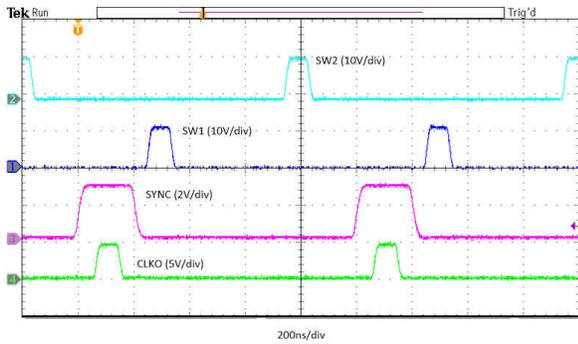
图 8-27. Sync In to SW1 and SW2 Delay
