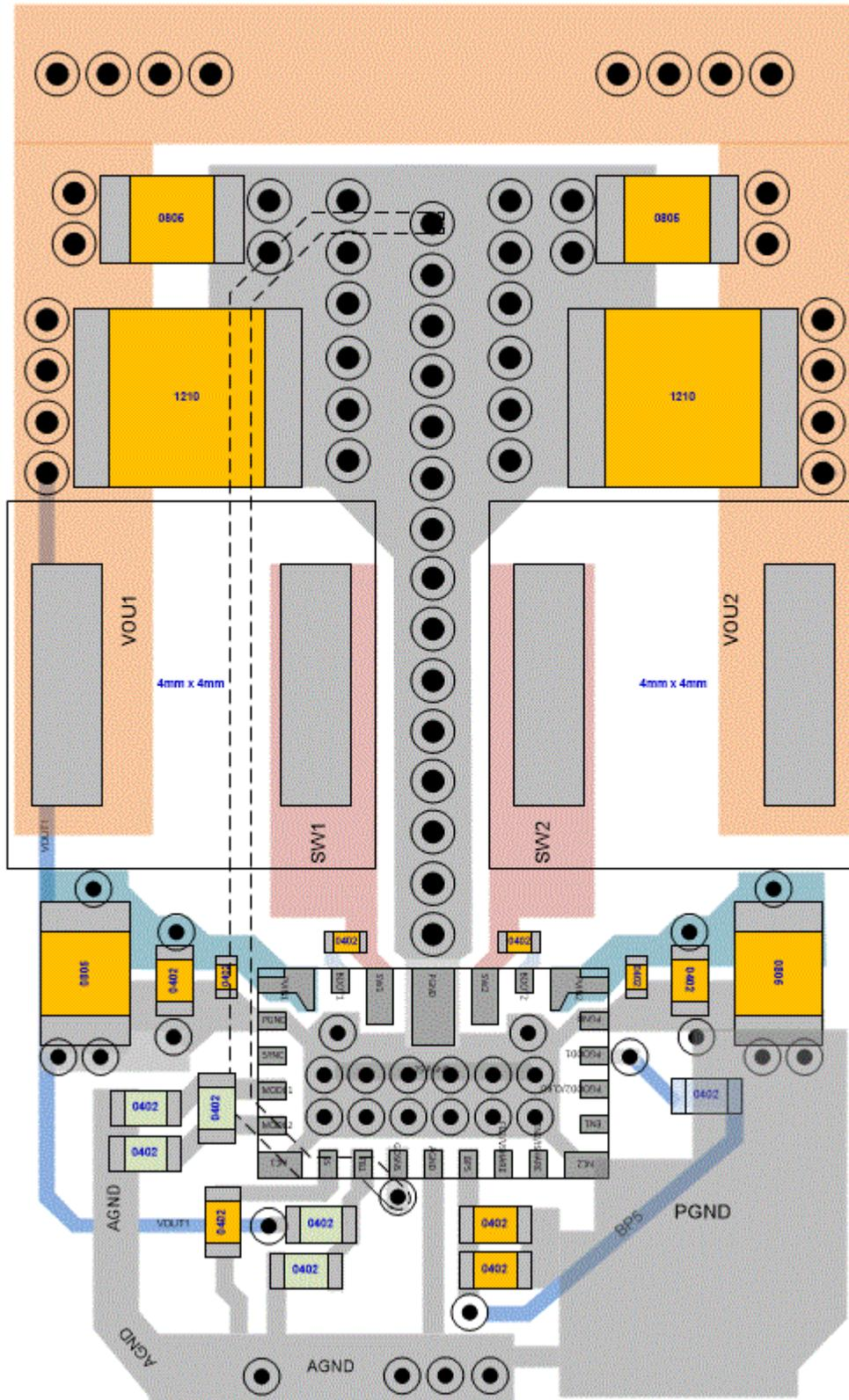
图 10-2. Example PCB Layout for Dual-phase Configuration
