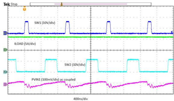
图 8-30. Input Ripple PVIN1 - 6-A Load
