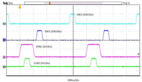
图 8-49. Sync In to SW1, SW2 and CLKO Delay
