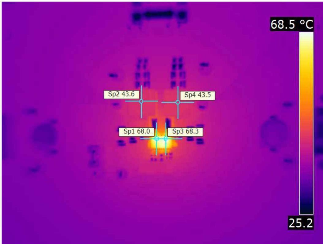
图 10-3. Thermal Image at 25°C Ambient - 2-phase Operation,  $f_{sw} = 1$  MHz,  $V_{IN} = 12$  V,  $V_{OUT} = 1$  V,  $I_{OUT} = 12$  A, Inductor = 560 nH (3.3 m $\Omega$  typical)
