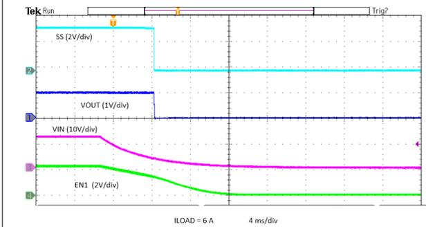
图 8-44. Power Down with  $V_{IN}$
