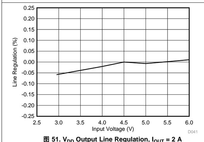
图 51.  $V_{DD}$  Output Line Regulation,  $I_{OUT} = 2\text{A}$
