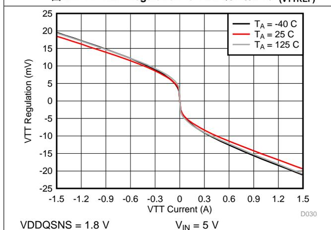
图 29. VTT Regulation to VTTREF vs I(VTT)
