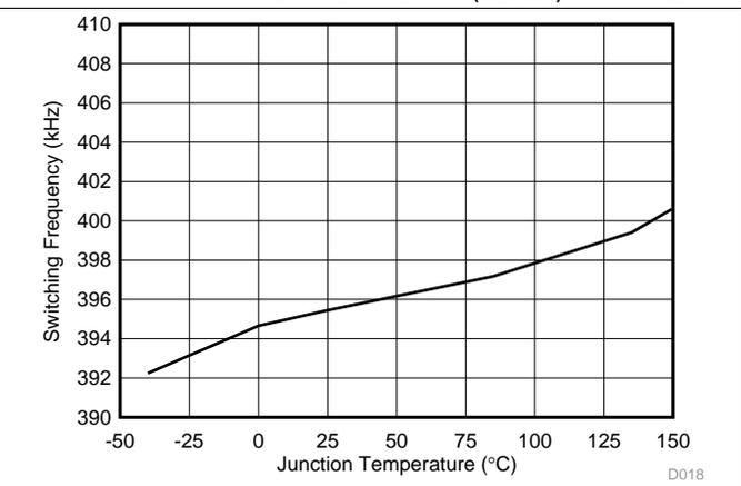
图 18. Switching Frequency vs Temperature
