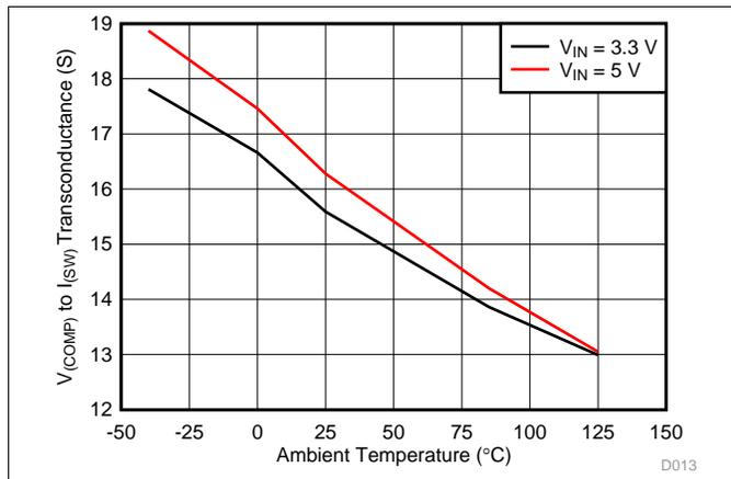
图 13.  $V_{COMP}$  to  $I_{SW}$  Transconductance vs Temperature
