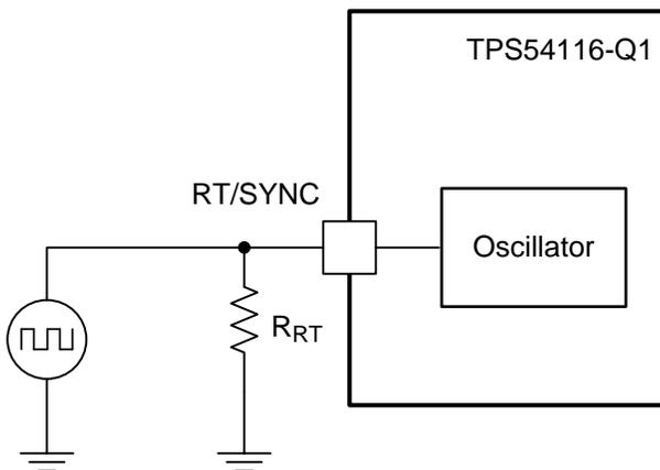
图 43. Synchronizing to a High Impedance System Clock
