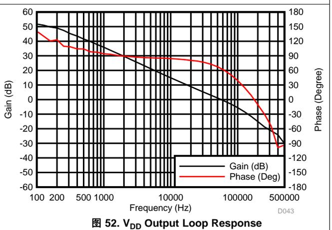
图 52.  $V_{DD}$  Output Loop Response
