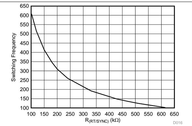
图 16. Switching Frequency vs  $R_{RT/SYNC}$  Low Range
