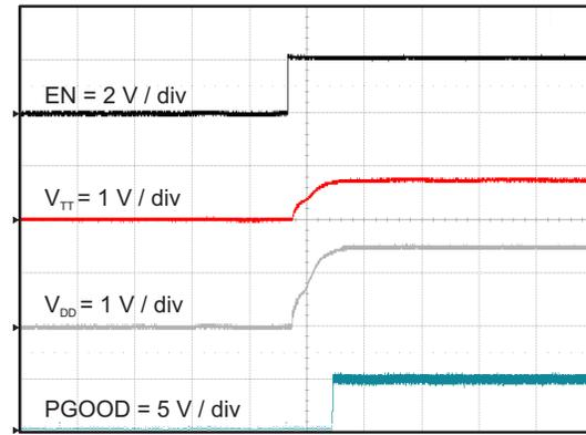
图 54.  $V_{TT}$  and  $V_{DD}$  Start-Up Relative to Enable
