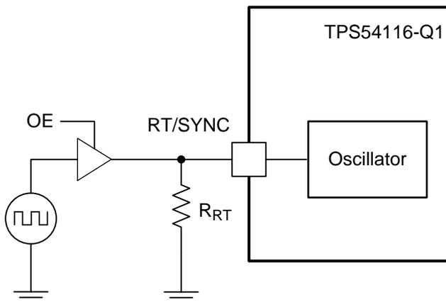
图 44. Interfacing to the RT/SYNC Pin with Buffer
