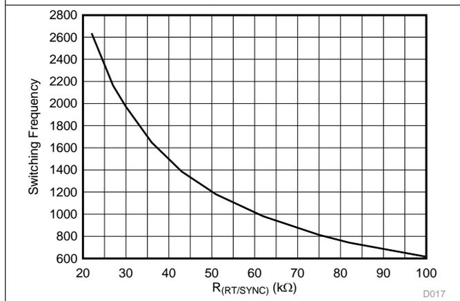
图 17. Switching Frequency vs  $R_{RT/SYNC}$  High Range
