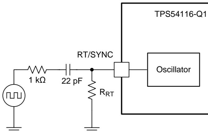
图 45. Interfacing to the RT/SYNC Pin with RC
