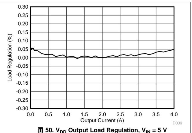
图 50.  $V_{DD}$  Output Load Regulation,  $V_{IN} = 5\text{V}$
