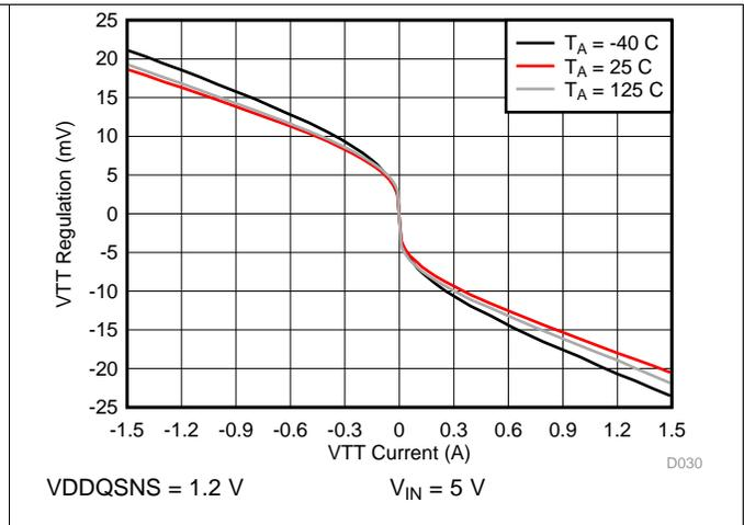
图 32. VTT Regulation to VTTREF vs I(VTT)
