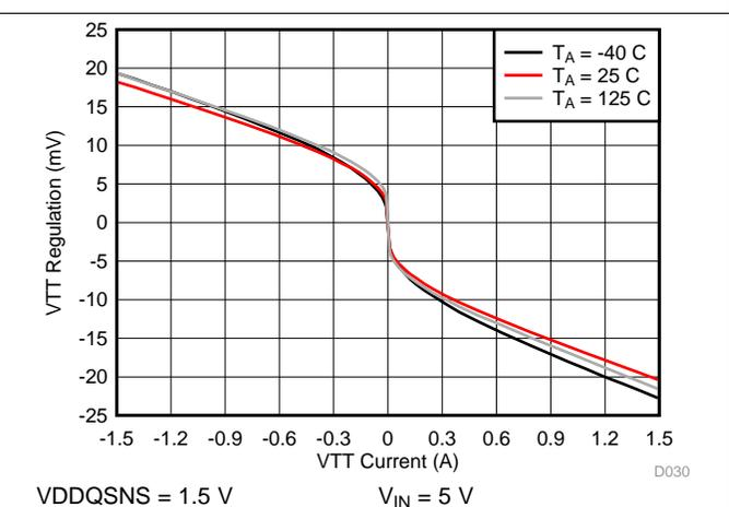
图 30. VTT Regulation to VTTREF vs I(VTT)
