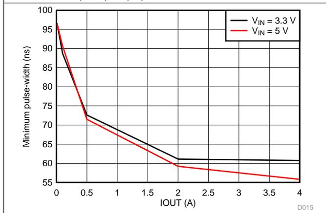
图 15. Minimum pulse-width vs Load Current
