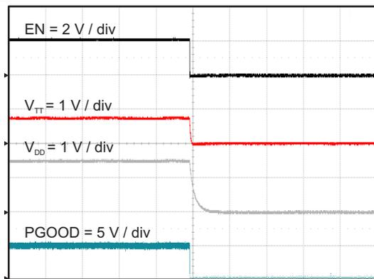
图 57.  $V_{TT}$  and  $V_{DD}$  Shutdown Relative to Enable
