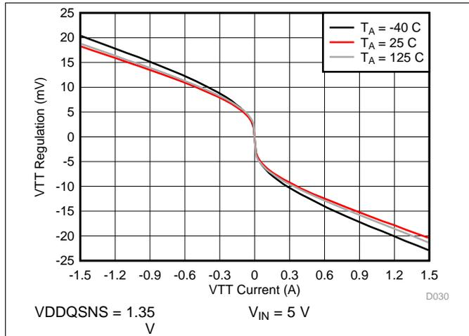
图 31. VTT Regulation to VTTREF vs I(VTT)
