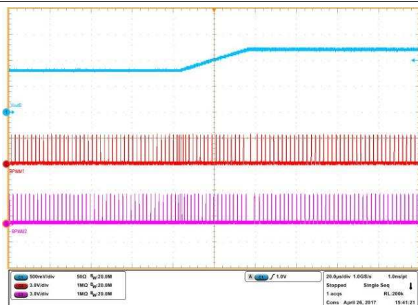
V_{VIN} = 12\text{ V} I_{OUT\_B} = 30\text{ A} V_{OUT\_B} VID step from 0.8 V to 1.2 V
