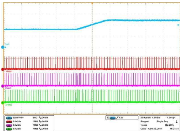
V_{VIN} = 12\text{ V} I_{OUT\_A} = 30\text{ A} V_{OUT\_A} VID step from 0.8 V to 1.2 V
