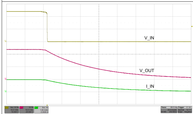
Figure 56. Start-Up With VIN—48-Ω Load
