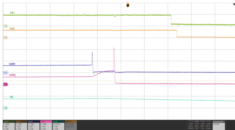
图 8-9. Parallel Devices Load Current During Steady State and Overload
