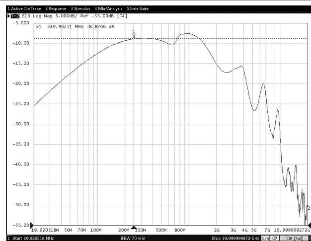
图 8-24. Off-state Data-Switch Isolation vs Frequency
