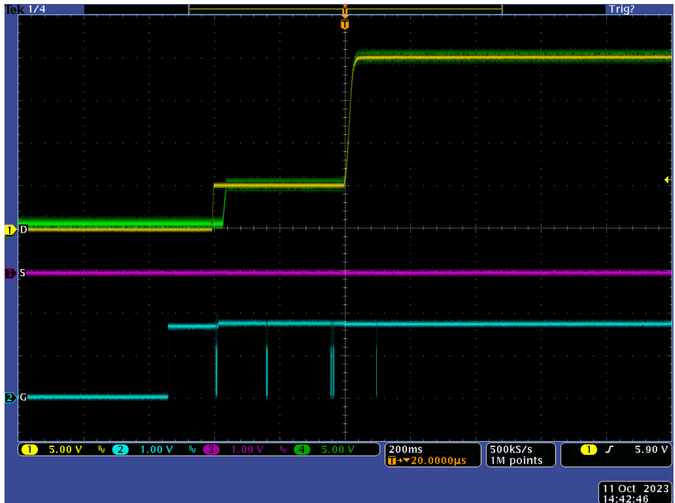
图 9-10. 20V PD Contract VBUS & PPHV (1-VBUS, 2-CC1, 3-CC2, 4-PPHV)
