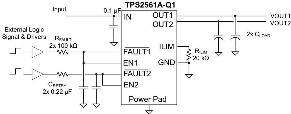
Figure 15. Auto-Retry Functionality With External EN Signal
