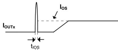
Figure 10. Response Time to Short Circuit Waveform
