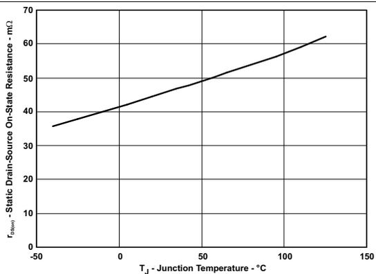
Figure 5. MOSFET  $r_{DS(on)}$  Vs. Junction Temperature
