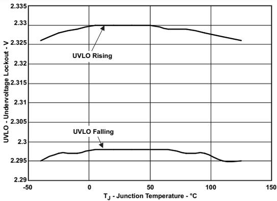
Figure 1. UVLO – Undervoltage Lockout – V
