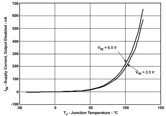
Figure 2.  $I_{IN}$  – Supply Current, Output Disabled – nA
