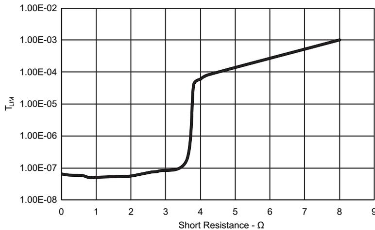
Figure 11. Overcurrent Response Time vs Short Resistance
