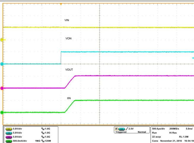
Figure 12. Rise Time  $t_R$  at  $V_{IN} = 5 V$
