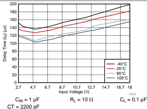
Figure 8. Delay Time ( $t_D$ ) vs Input Voltage
