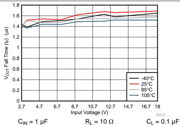
Figure 9.  $V_{OUT}$  Fall Time ( $t_F$ ) vs Input Voltage
