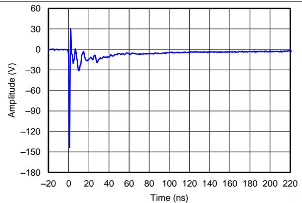
**Figure 4. IEC 61000-4-2 Clamping Voltage, -8-kV Contact**
