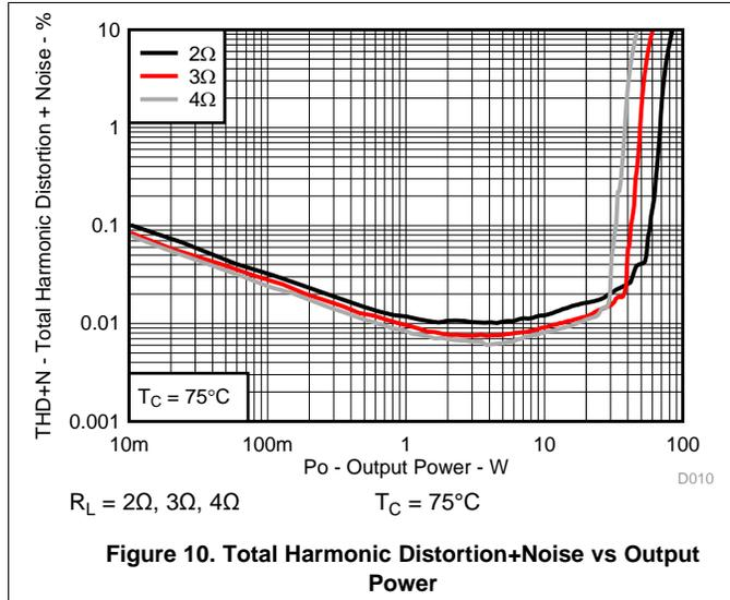
**Figure 10. Total Harmonic Distortion+Noise vs Output Power**
