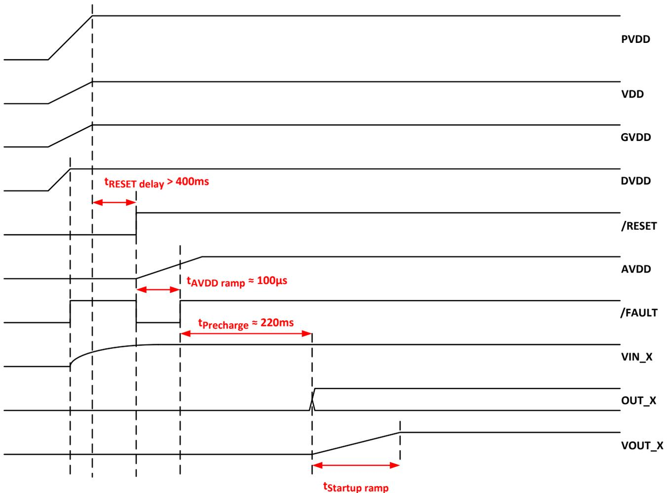
**Figure 28. Startup Timing**
