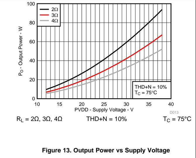
**Figure 13. Output Power vs Supply Voltage**
