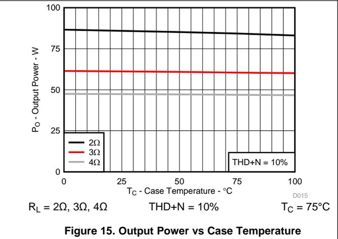
**Figure 15. Output Power vs Case Temperature**
