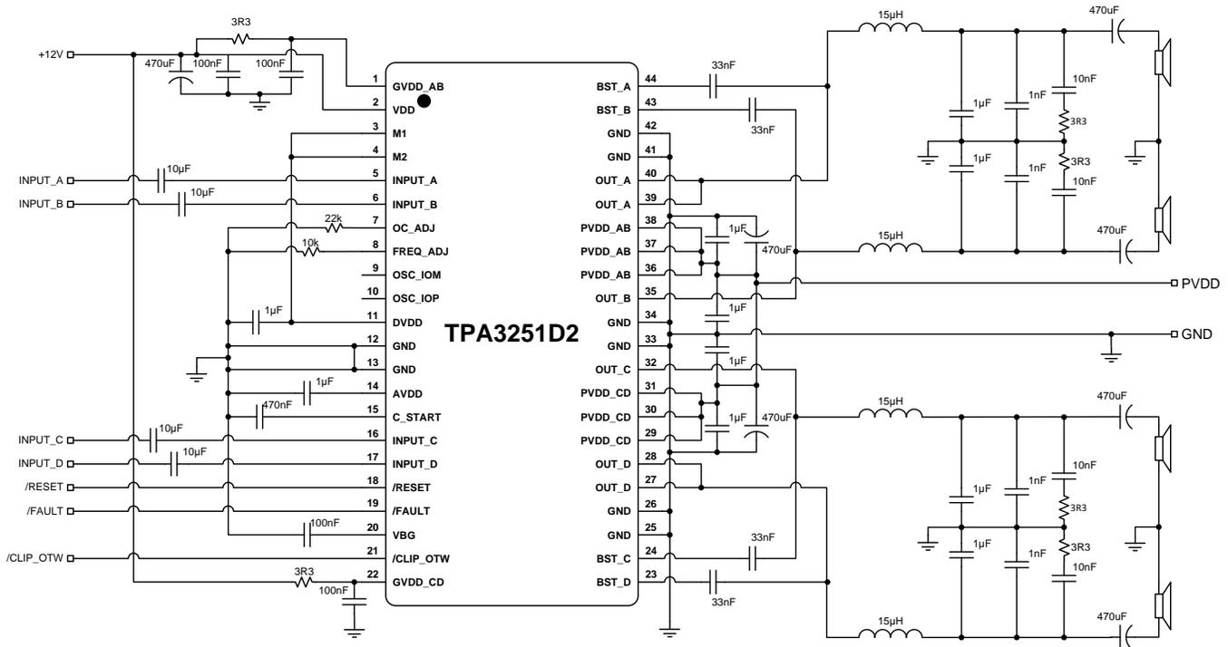
Figure 26. Typical Single Ended (1N) SE Application
