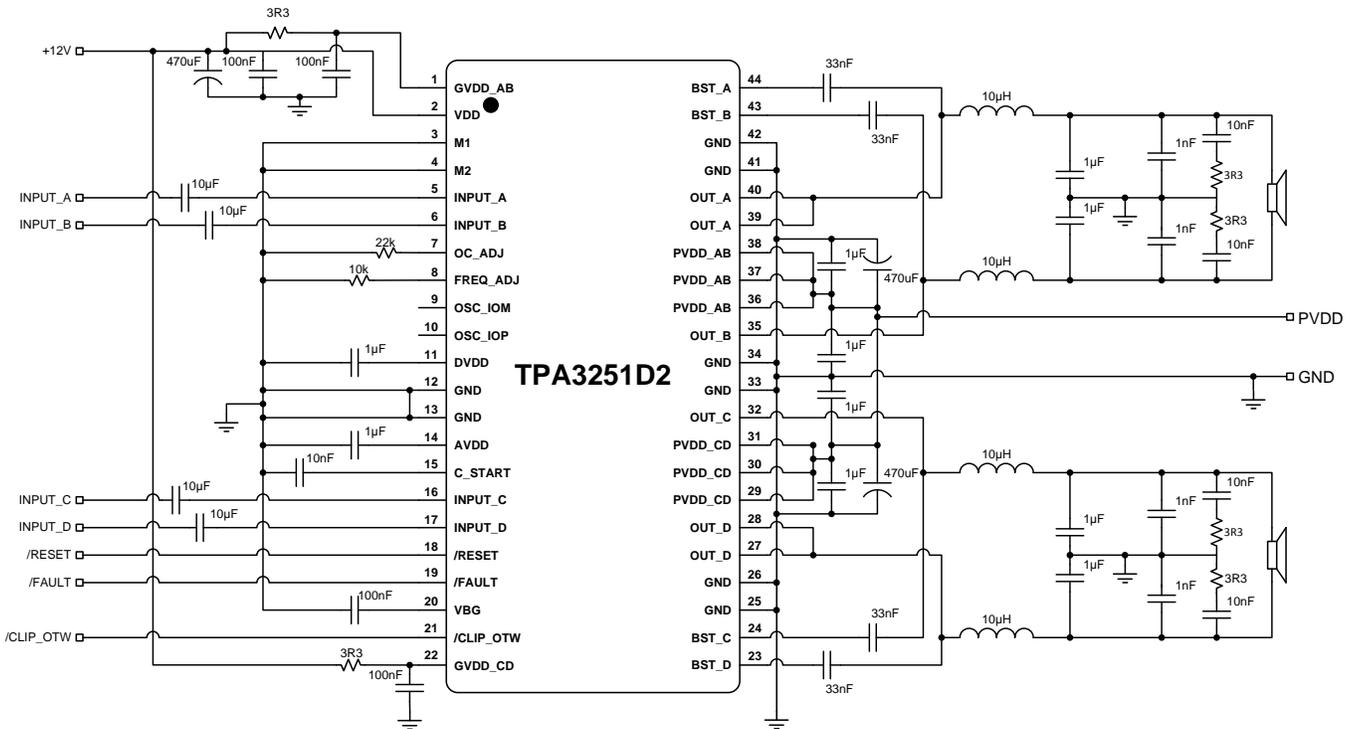
Figure 25. Typical Differential Input BTL Application
