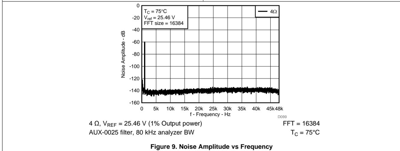
Figure 9. Noise Amplitude vs Frequency
