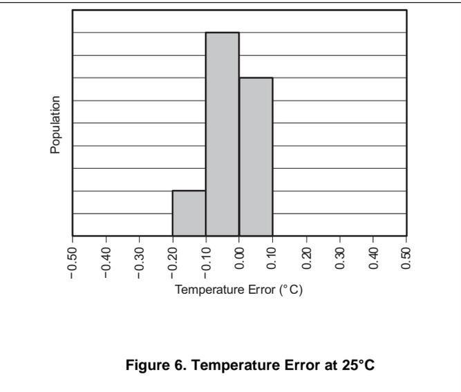
Figure 6. Temperature Error at 25°C
