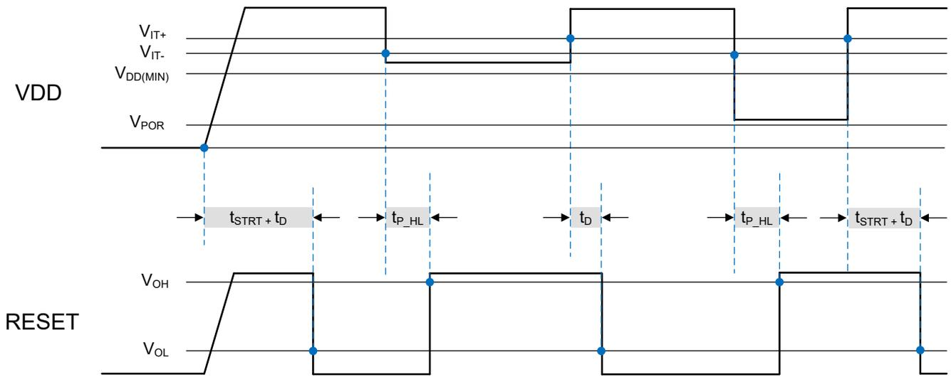
(6)  $t_{D (no\ cap)}$  is included in  $t_{STRT}$  time delay. If  $t_D$  delay is programmed by an external capacitor connected to CT pin then  $t_D$  programmed time will be added to the startup time, VDD slew rate = 100 mV /  $\mu$ s.
