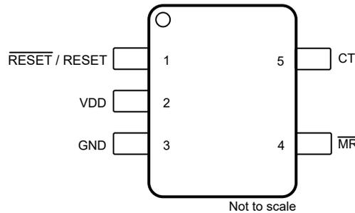
**Figure 6-1. Pin Configuration TLV840M-Q1
