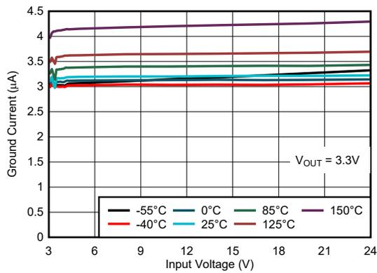
图 6-15. Ground Pin Current vs Input Voltage for New Chip
