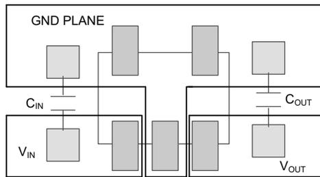
**图 8-8. Layout Example for the DBV Package**
