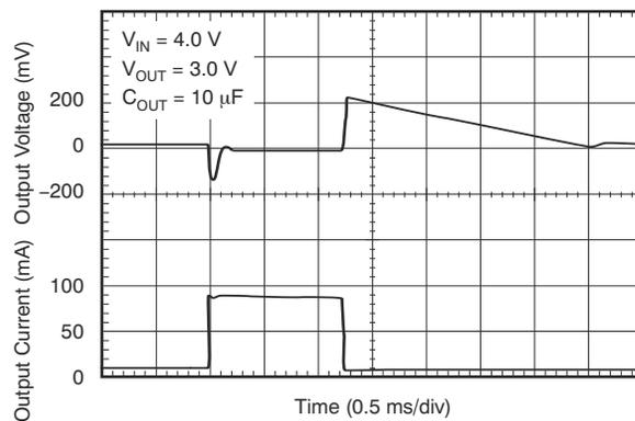
图 6-24. Load Transient Response for Legacy Chip
