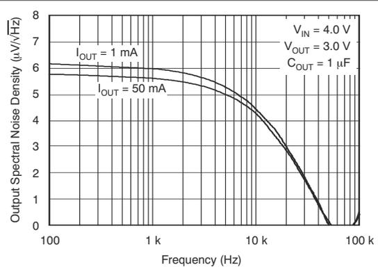
图 6-18. Output Spectral Noise Density vs Frequency for Legacy Chip
