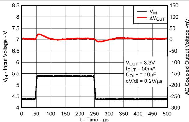
图 6-23. Line Transient Response for New Chip
