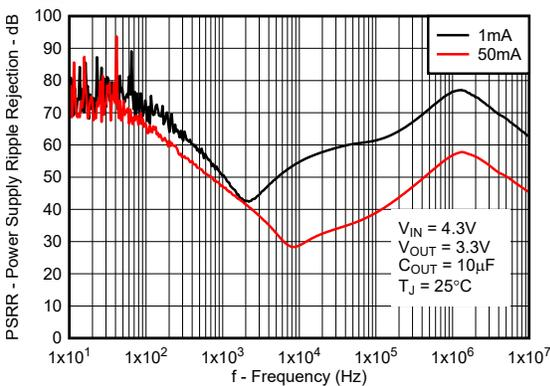
图 6-21. Power-Supply Ripple Rejection vs Frequency for New Chip
