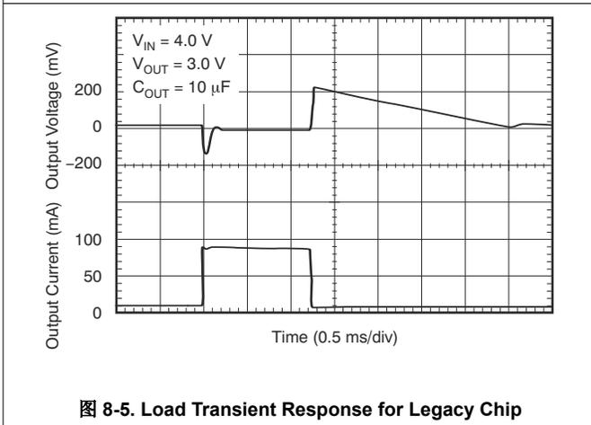
图 8-5. Load Transient Response for Legacy Chip
