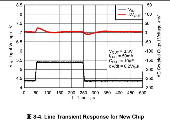
图 8-4. Line Transient Response for New Chip
