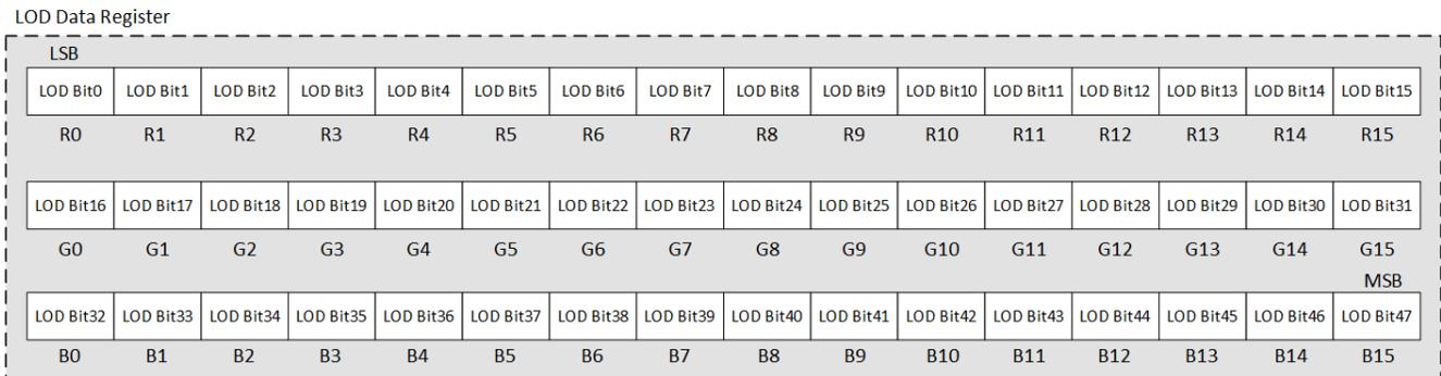
图 8-9. Bit Arrangement in LOD Data Register
