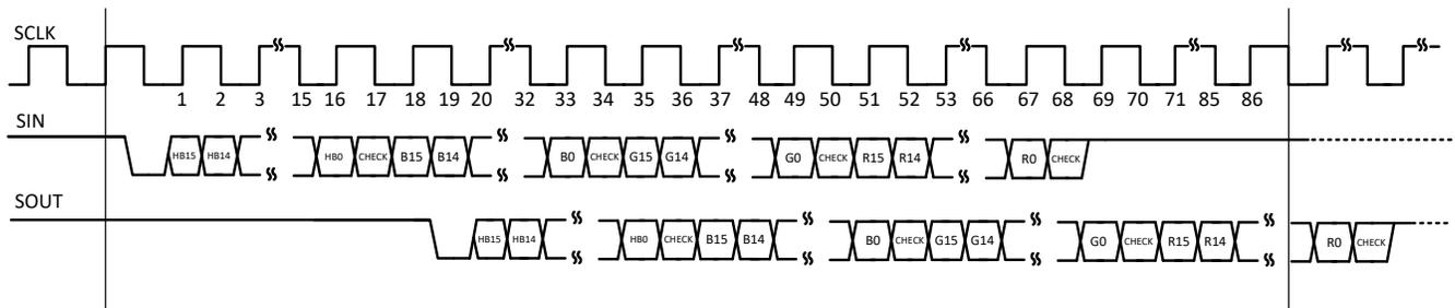
图 8-22. Data Write Command with Broadcast (Timing Diagram)
