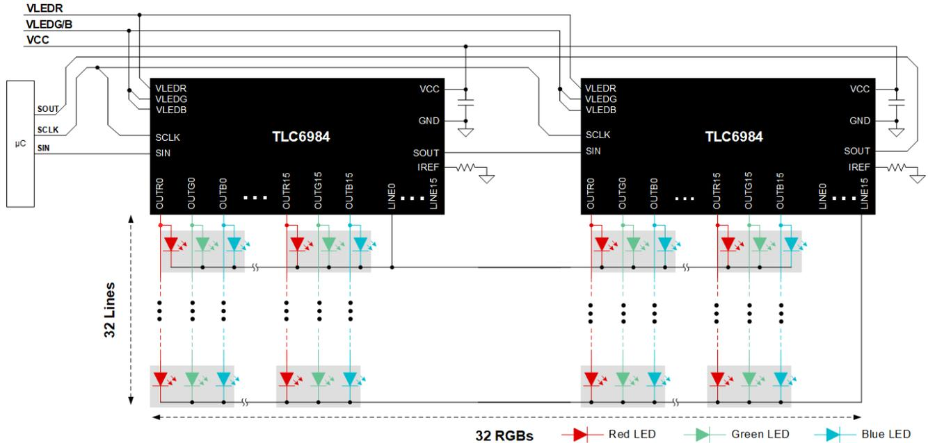
图 9-1. TLC6984 With Dual Devices Stackable Connection
