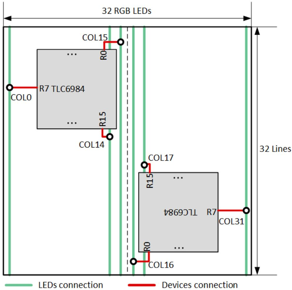
图 11-3. Channel Routing Suggestion With Shortest Wire
