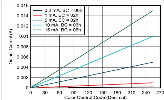
图 7-6. Color Control Code vs Output Current
