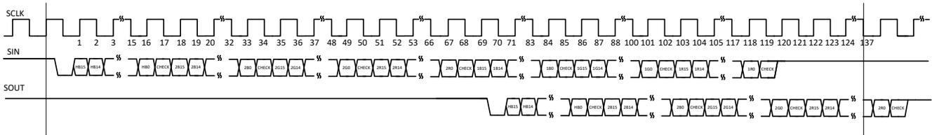
图 8-24. Data Write Command with Non-Broadcast (Timing Diagram)
