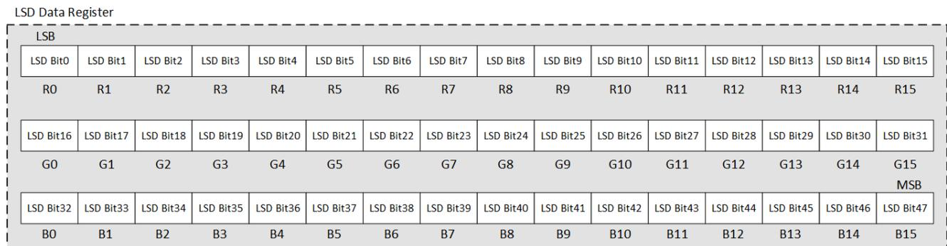
图 8-13. Bit Arrangement in the LSD Data Register
