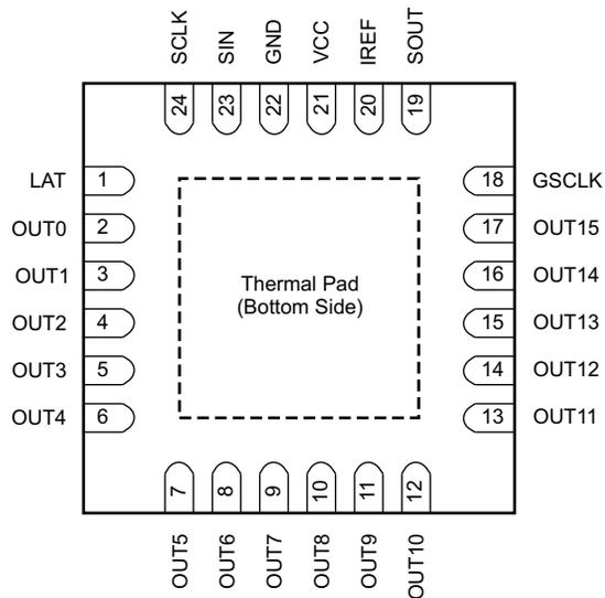
NOTE: The thermal pad is not internally connected to GND. The thermal pad must be connected to GND via the printed board circuit (PCB) pattern.
