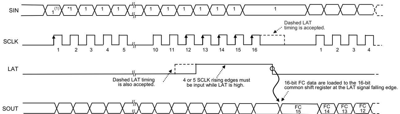
**Figure 24. FC Data Read (READFC) Command Timing Diagram**
