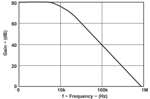
**Figure 7-4. Error Amplifier Bode Plot**
