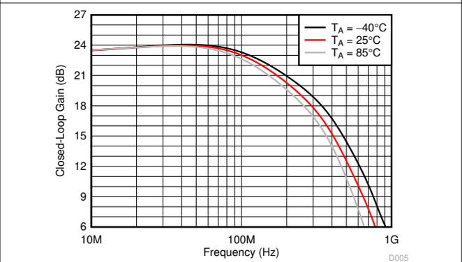
图 5-4. Small-Signal Frequency Response vs Temperature
