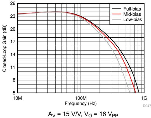
图 5-15. Large-Signal Frequency Response vs Bias Modes
