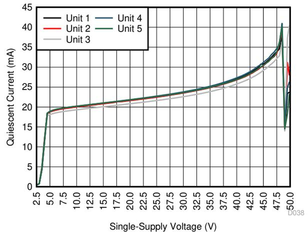
**图 6-6. Typical Device Breakdown Supply Voltage ( $T_A = 27^\circ\text{C}$ )**
