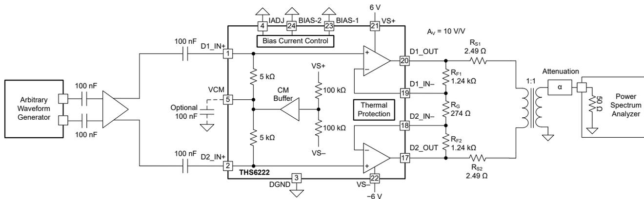
图 7-2. Measurement Test Circuit for Out-of-Band Suppression
