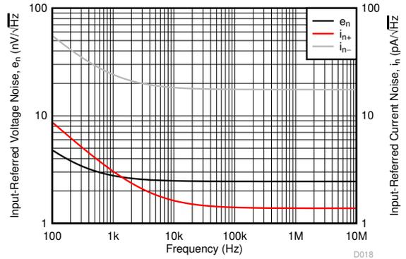
图 5-16. Input Voltage and Current Noise Density vs Frequency
