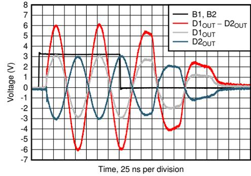
**图 5-36. Full-Bias and Shutdown Mode Transition Timing**
