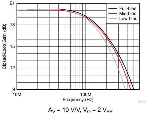
图 5-13. Small-Signal Frequency Response vs Bias Modes
