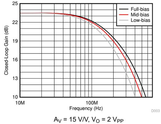
图 5-14. Small-Signal Frequency Response vs Bias Modes
