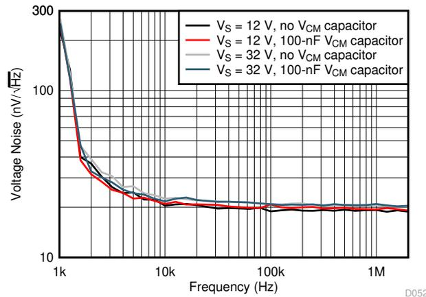
图 6-1. Common-Mode Voltage Noise Density vs Frequency
