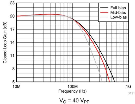
图 5-41. Large-Signal Frequency Response vs Bias Modes
