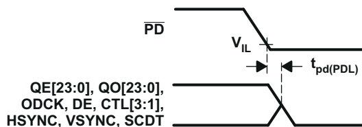
图 8-7. Delay From \overline{PD} Low to Hi-Z Outputs
