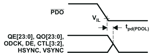
图 8-8. Delay From \overline{PDO} Low to Hi-Z Outputs
