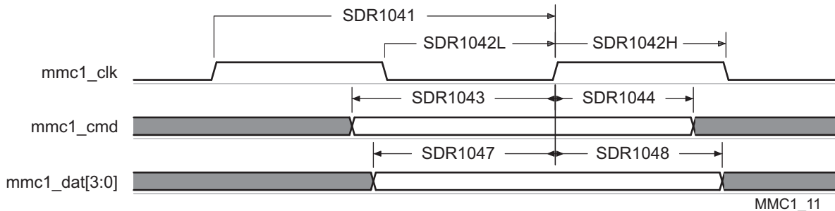
Figure 5-80. MMC/SD/SDIO in - High Speed SDR104 - Receiver Mode
