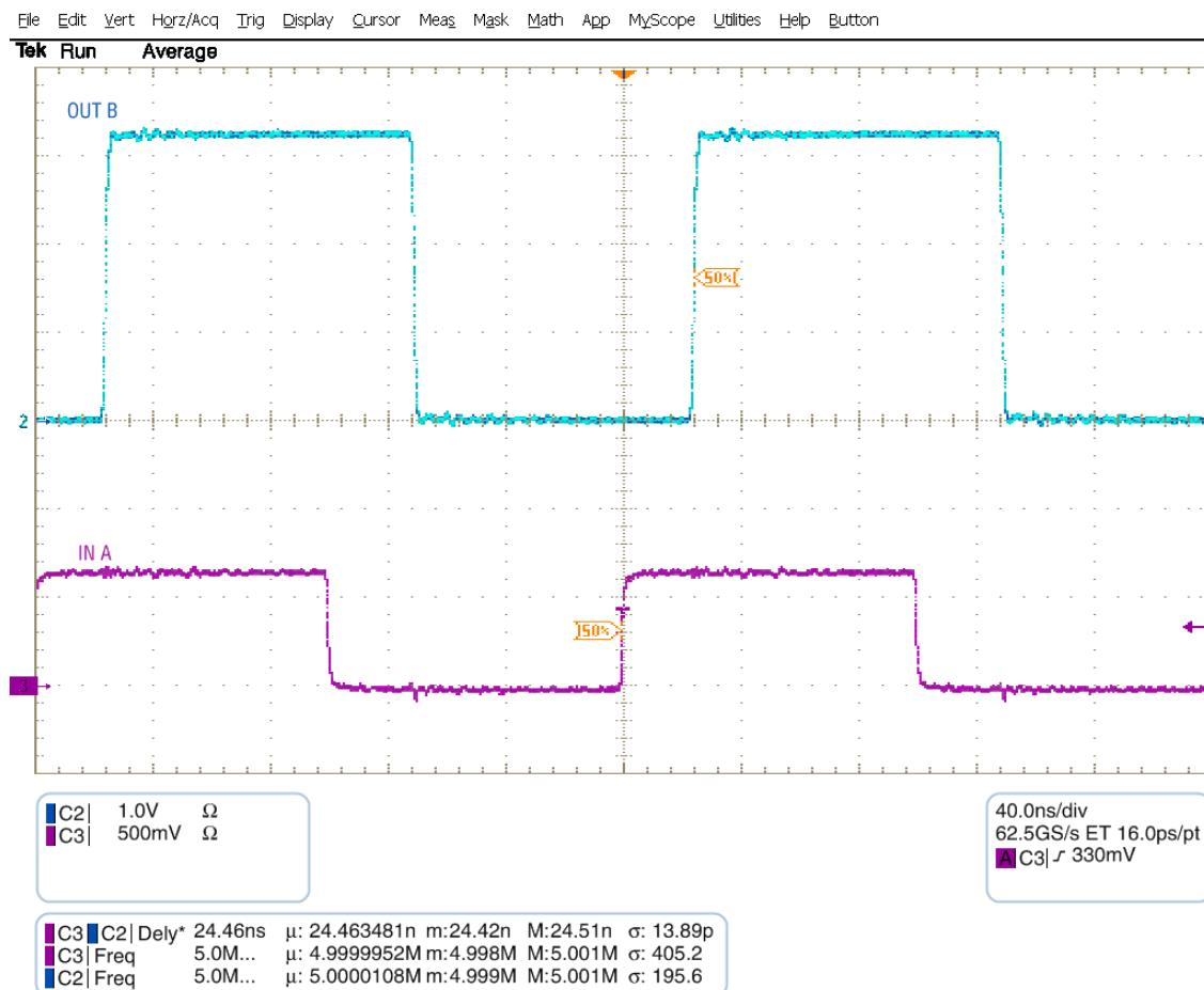
**图 9-2. Up Translation at 2.5 MHz (0.7 V to 3.3 V)**
