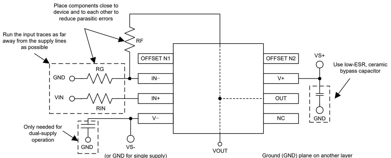
图 8-7. Operational Amplifier Board Layout for Noninverting Configuration
