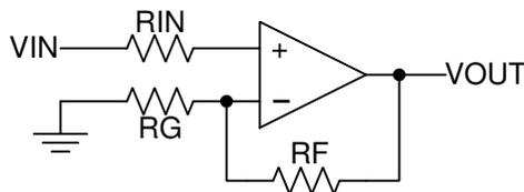
图 8-6. Operational Amplifier Schematic for Noninverting Configuration
