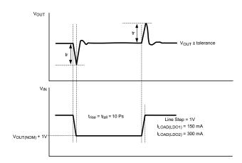
Figure 3. Line Transient Input Test Signal
