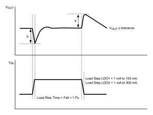
Figure 4. Load Transient Input Signal
