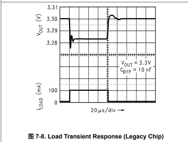
图 7-8. Load Transient Response (Legacy Chip)
