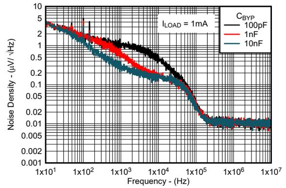
图 5-22. Output Noise Density vs Frequency (New Chip)
