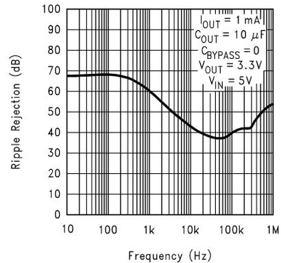
图 5-6. Ripple Rejection vs Frequency (Legacy Chip)
