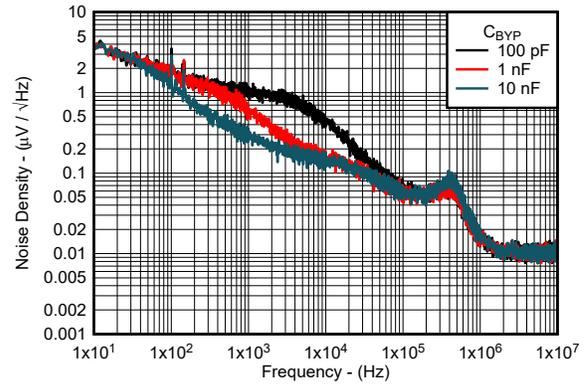
图 5-20. Output Noise Density vs Frequency (New Chip)
