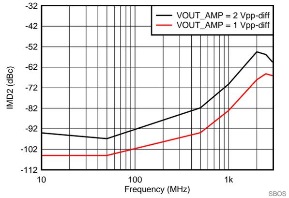
图 47. SE-DE 2nd Order Intermodulation Distortion vs Frequency
