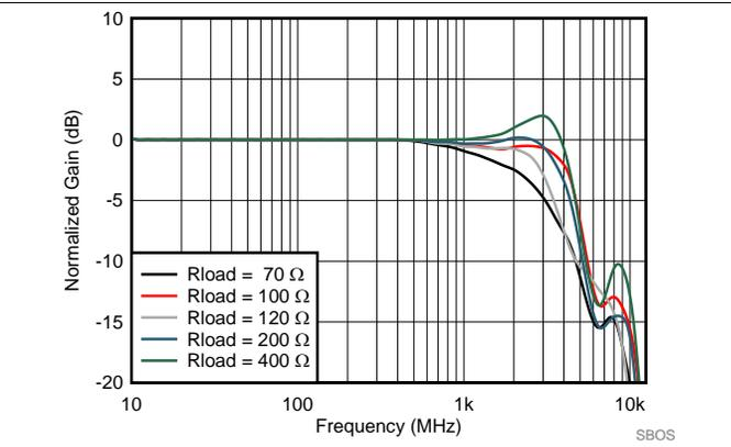
图 35. SE-DE Small Signal Frequency Response vs Rload
