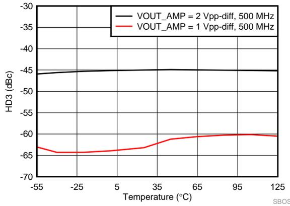
图 46. SE-DE 3rd Order Harmonic Distortion vs Temperature
