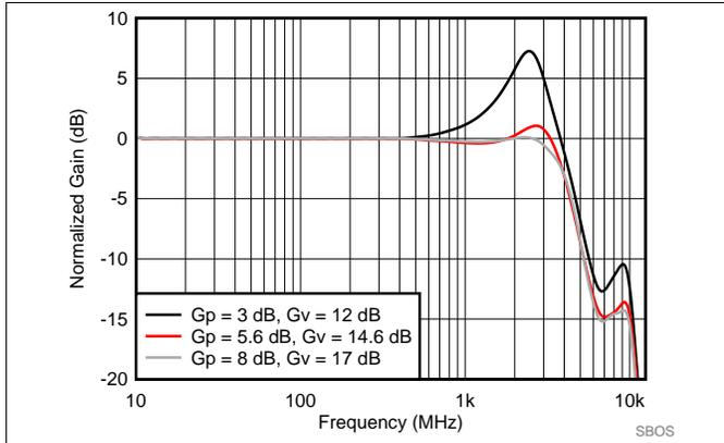
图 34. SE-DE Small Signal Frequency Response vs Gain
