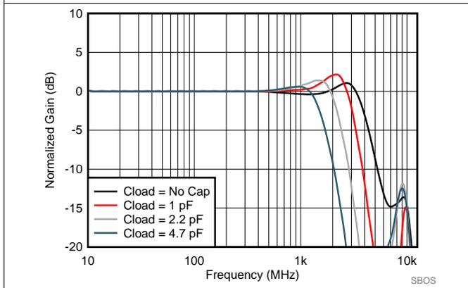
图 36. SE-DE Small Signal Frequency Response vs Cload
