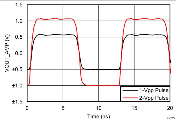
**图 30. SE-DE Output Signal Pulse Response**
