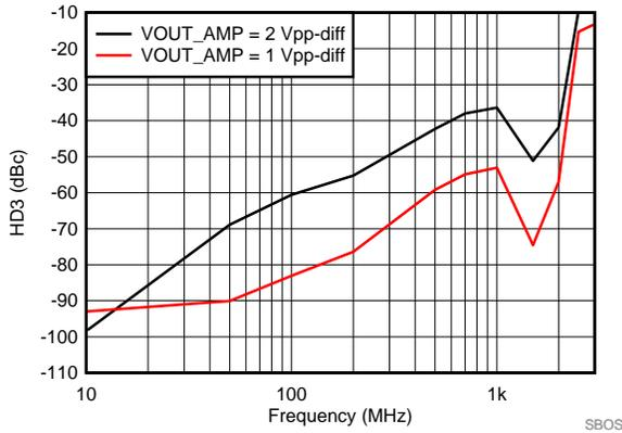
图 40. SE-DE 3rd Order Harmonic Distortion vs Frequency
