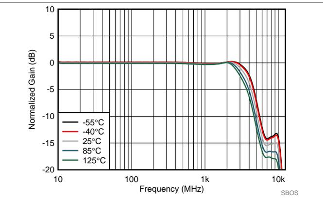
图 37. SE-DE Small Signal Frequency Response vs Temperature
