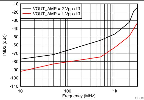
图 48. SE-DE 3rd Order Intermodulation Distortion vs Frequency
