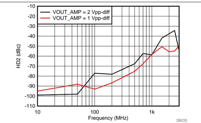
图 39. SE-DE 2nd Order Harmonic Distortion vs Frequency
