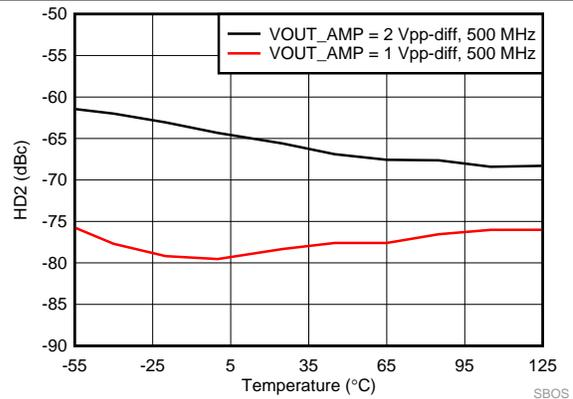
图 45. SE-DE 2nd Order Harmonic Distortion vs Temperature
