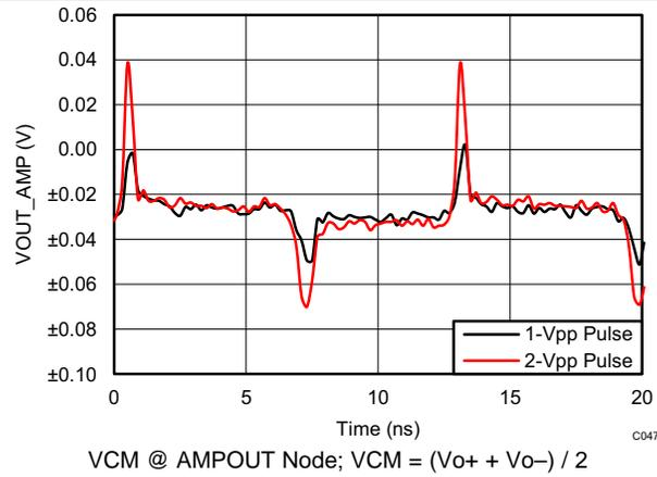
图 52. SE-DE Output Common Mode Pulse Response
