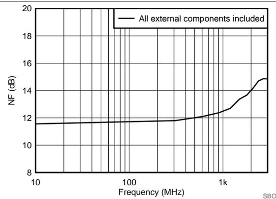
**图 29. SE-DE Noise Figure vs Frequency**
