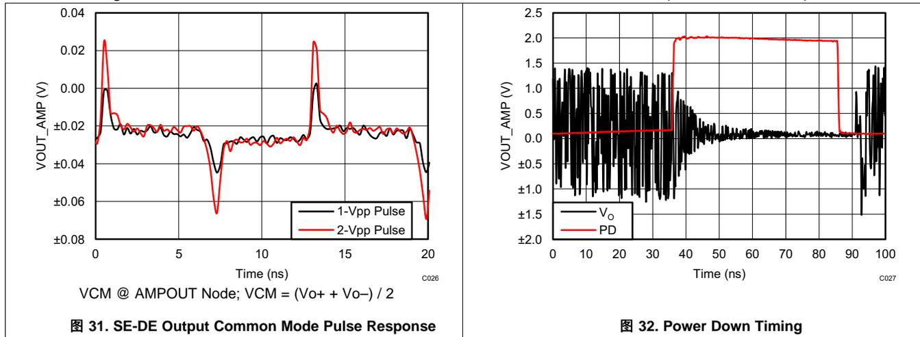
图 31. SE-DE Output Common Mode Pulse Response
