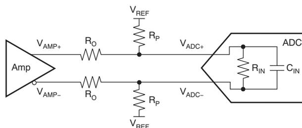
**图 69. Resistor Network to DC Level-Shift Common-Mode Voltage**
