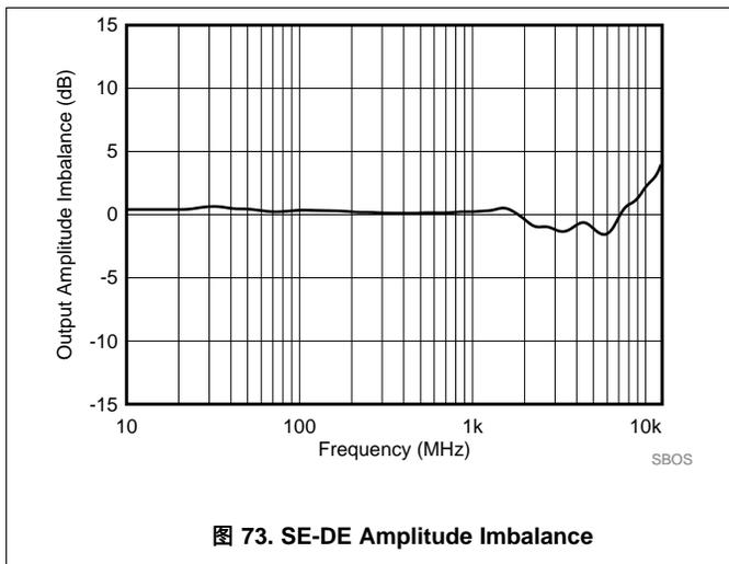
图 73. SE-DE Amplitude Imbalance
