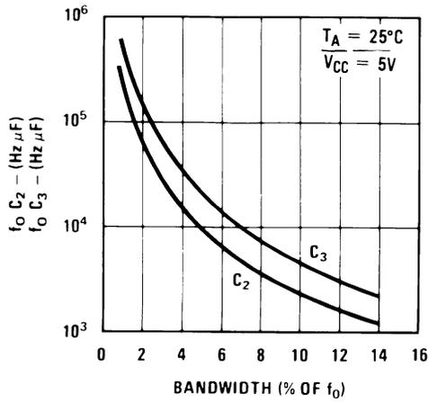
图 7-7. Detection Bandwidth as a Function of  $C_2$  and  $C_3$
