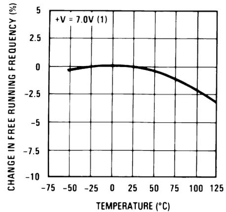
图 7-4. Typical Frequency Drift
