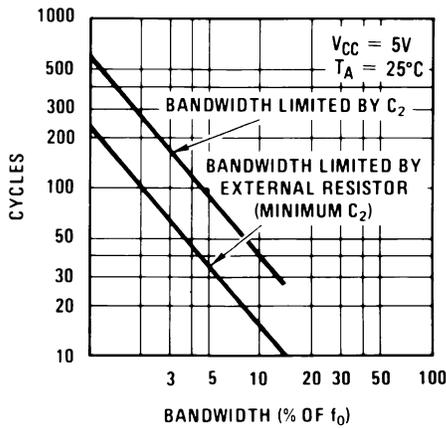
图 7-9. Greatest Number of Cycles Before Output
