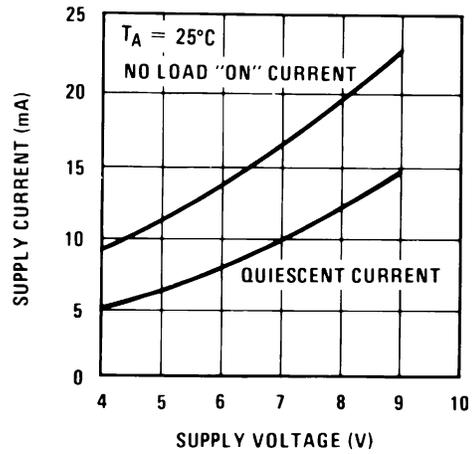
图 7-8. Typical Supply Current vs Supply Voltage
