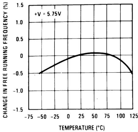
图 7-1. Typical Frequency Drift
