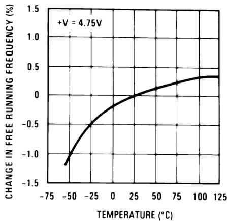
图 7-3. Typical Frequency Drift
