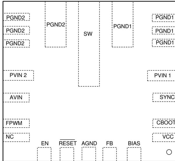
图 6-1. RNL Package 22-Pin VQFN Top View
