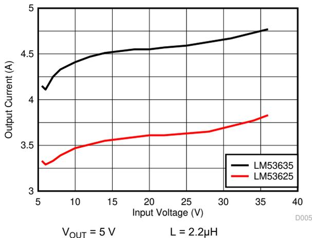
图 9-15. Output Current Level Limit Before Overcurrent Protection
