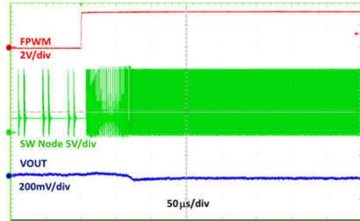
$V_{OUT} = 3.3\text{ V}$   $I_{OUT} = 10\text{ mA}$
