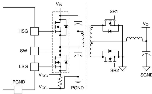
图 7-11. Half-Bridge Converter with Low-Side Current Sensing
