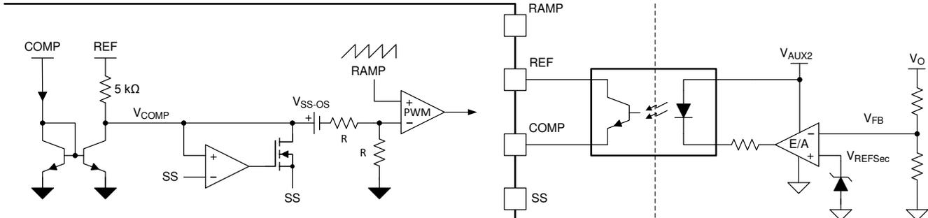
**图 7-2. Voltage-Mode Feedback Control Loop for Half-Bridge Converter**
