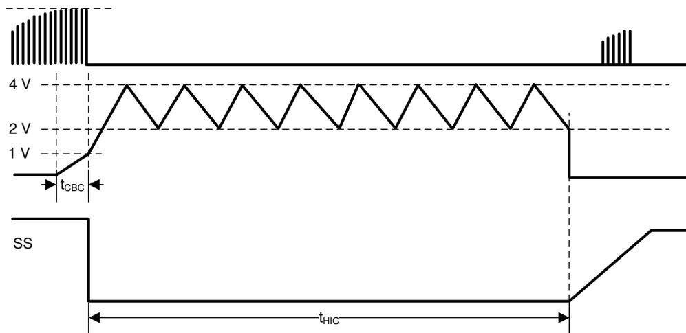
图 7-18. Hiccup Mode Activated By Continuous CBC Operation
