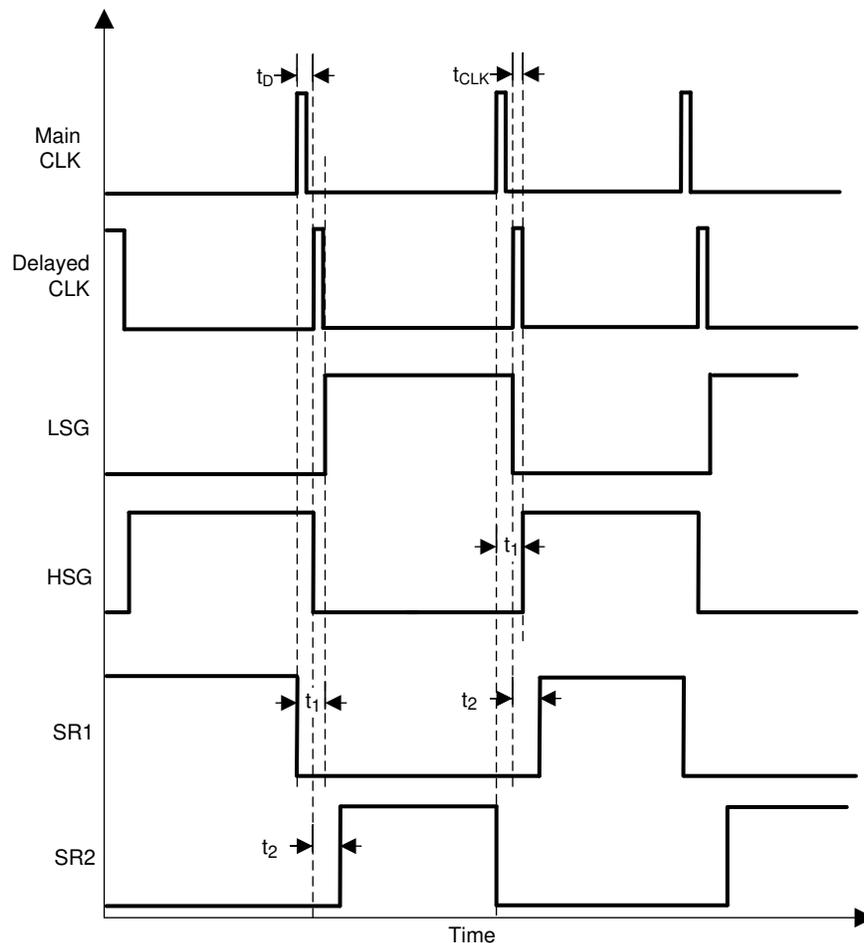
图 7-7. PWM Signals at Maximum Duty Cycle Condition
