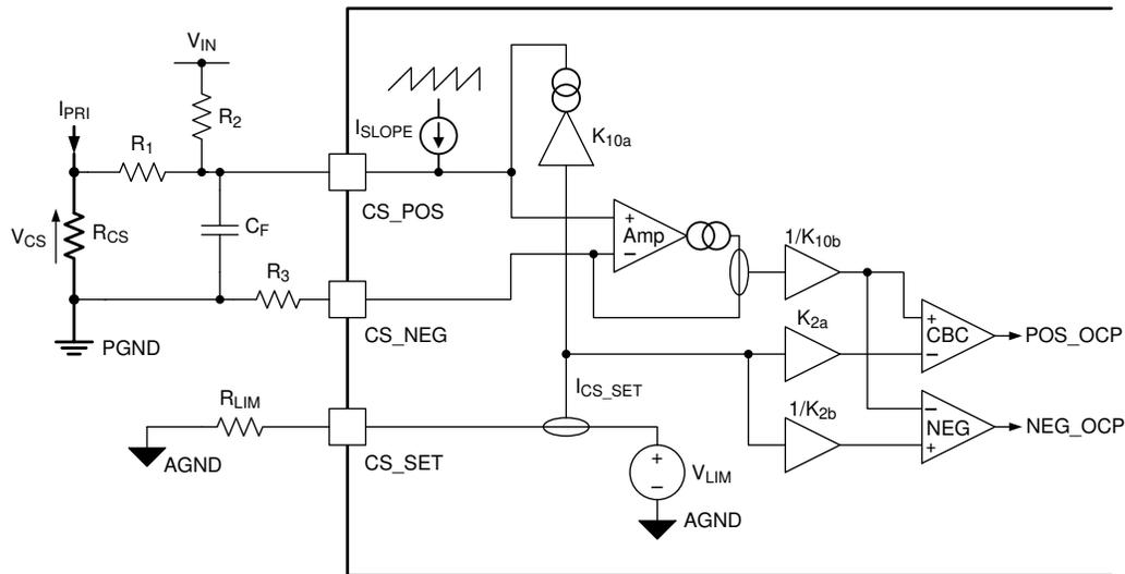
图 7-12. Block Diagram of the Current Limiting Function
