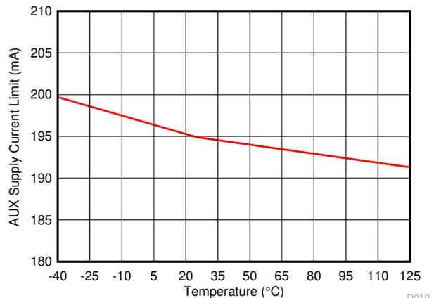
图 6-10. Auxiliary Supply Current Limit vs Temperature
