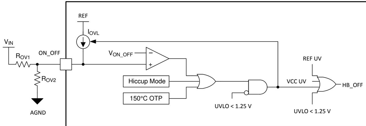
图 7-21. ON/OFF Pin Configured as OVP Pin
