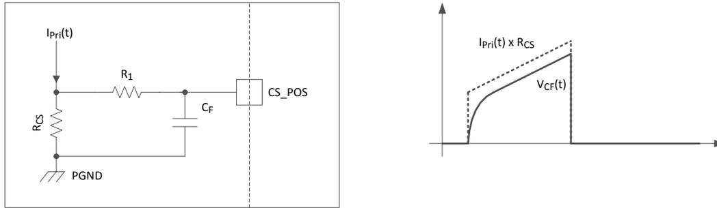
图 8-10. CS\_POS Filter Circuit Model and Waveform
