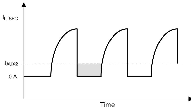
**图 8-11. Auxiliary Transformer Secondary Winding Current Waveforms for  $C_{\text{AUX2}}$  Ripple Calculation**
