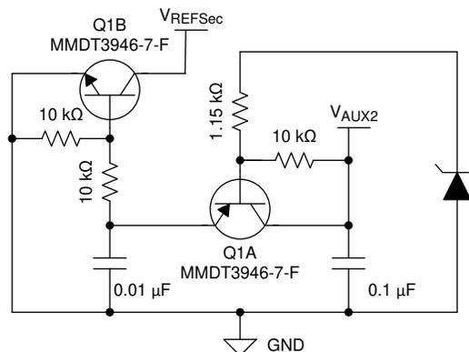
图 8-3. Secondary Auxiliary Voltage Level-Shift Detection Circuit
