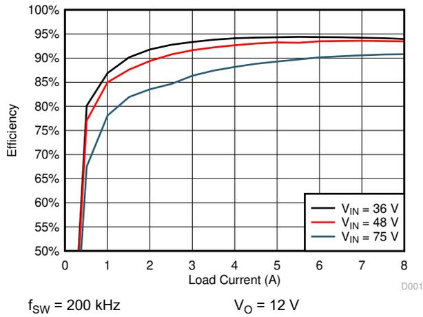
图 6-1. Application Board Efficiency vs Load Current
