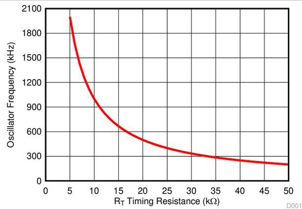
图 6-5. Oscillator Frequency vs  $R_T$  Timing Resistance
