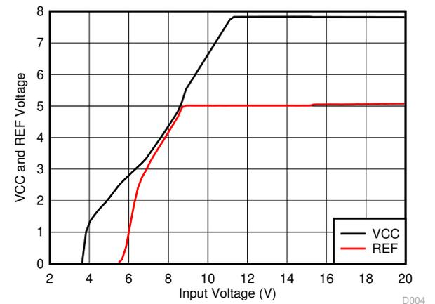
图 6-4. VCC and REF Voltage vs Input Voltage
