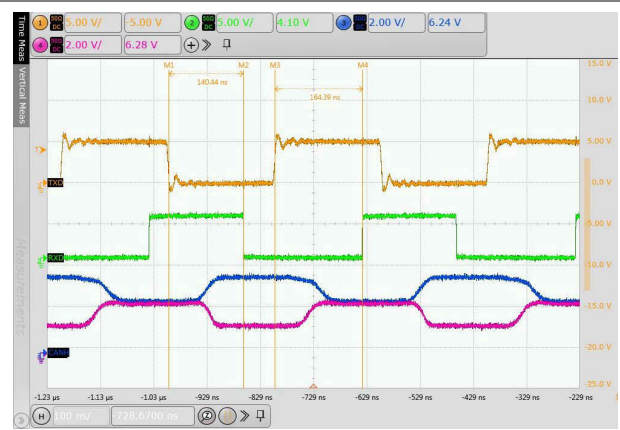
图 8-16. Typical TXD, RXD, CANH and CANL Waveforms at 5 Mbps
